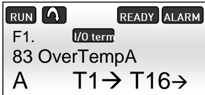
Figure 7.1-2, High temperature alarm on the NXP panel
