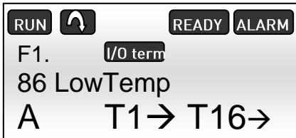
Figure 7.1-3, Low temperature alarm on the NXP panel
