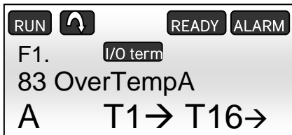
Figure 7.1-2, High temperature alarm on the NXP panel
