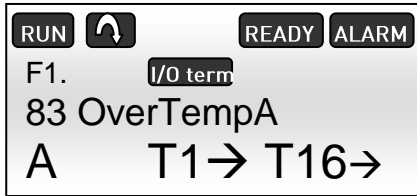
Figure 7.1-2, High temperature alarm on the NXP panel
