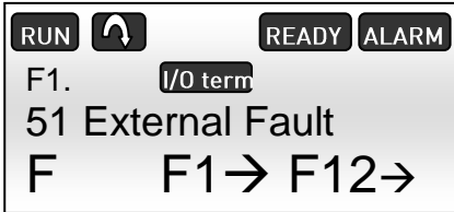
Figure 7.1-5, Leak alarm on the NXP panel
