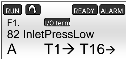
Figure 7.1-4, Low pressure alarm on the NXP panel
