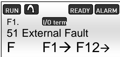
Figure 7.1-5, Leak alarm on the NXP panel
