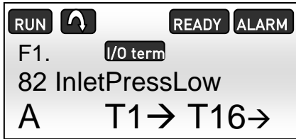
Figure 7.1-4, Low pressure alarm on the NXP panel
