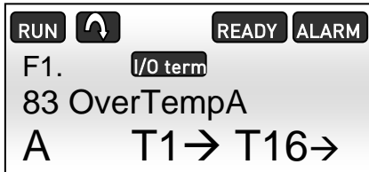
Figure 7.1-2, High temperature alarm on the NXP panel
