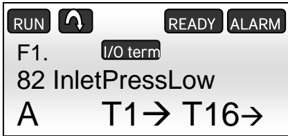
Figure 7.1-4, Low pressure alarm on the NXP panel
