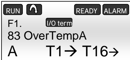
Figure 7.1-2, High temperature alarm on the NXP panel
