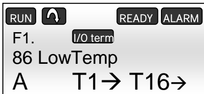
Figure 7.1-3, Low temperature alarm on the NXP panel
