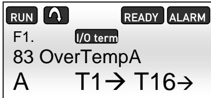
Figure 7.1-2, High temperature alarm on the NXP panel
