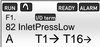
Figure 7.1-4, Low pressure alarm on the NXP panel
