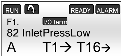
Figure 7.1-4, Low pressure alarm on the NXP panel
