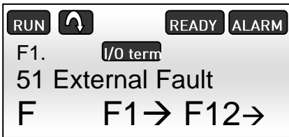
Figure 7.1-5, Leak alarm on the NXP panel
