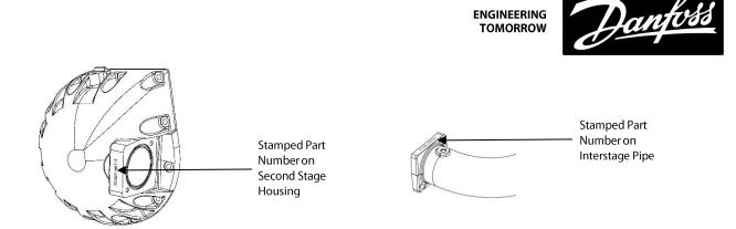
Note: Do not replace this pipe unless the numbers on the old and new Interstage Pipe match!
