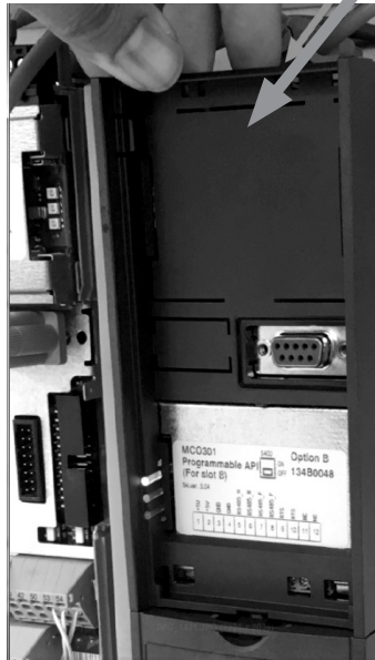
Carefully remove the plastic cover by unlocking the tab on the top of the drive and releasing.
