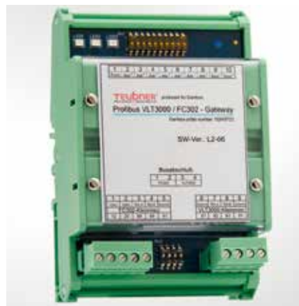
Upgrade without programming: VLT® 3000 SINEC L2 converter
