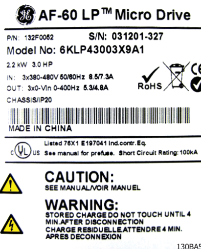
Illustration 2.1 This Example Shows the Nameplate Sticker
