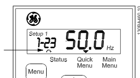
Figure 3.6 Indicating Motor Direction
