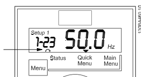
Illustration 7.7 Indicating Motor Direction
