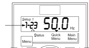
Illustration 7.4 Indicating Selected Parameter Number
