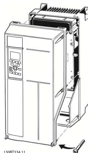
Illustration 2.14 Control Wiring Access for IP55 / Nema 12 enclosures
