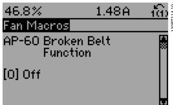
Illustration 6.5 Step 4: Use the up/down navigation keys to scroll down to find AP-62 Broken Belt Delay.
