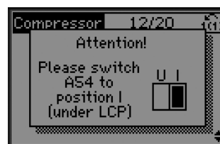
Figure 3.14 Info: Set Switch Accordingly
