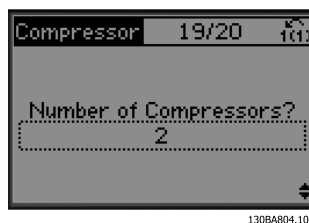
Figure 3.21 Set Number of Compressors in Pack
