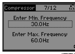
Illustration 4.7 Min. and Max. Frequency Set-up
