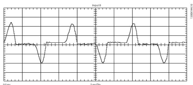
**Illustration 6.17 Input Current Waveform with Phase Loss**
