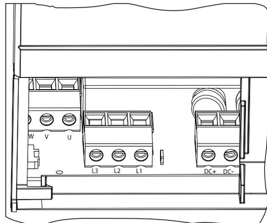
Illustration 6.10 UDC Terminals Location on H9 Frequency Converter
