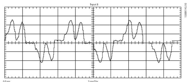
**Illustration 6.16 AC Input Current Waveform with Diode Bridge**
