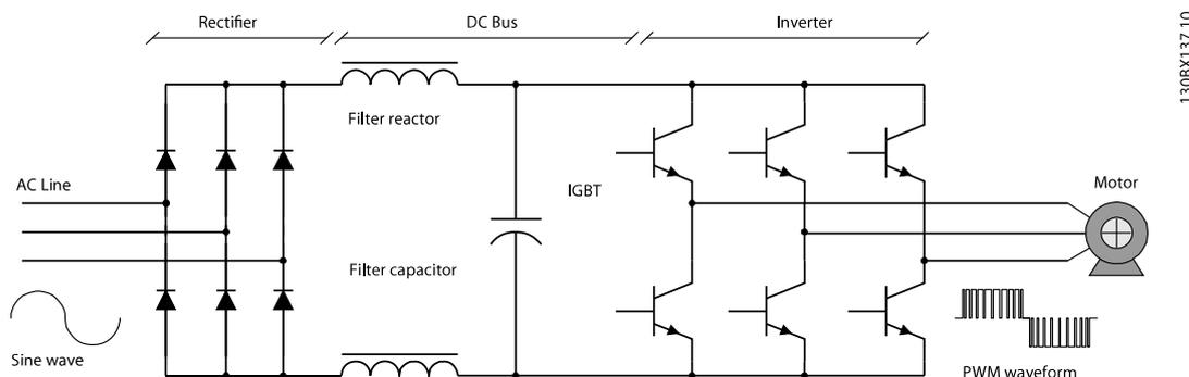
Illustration 5.1 Frequency Converter Functionality Diagram
