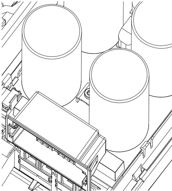
Illustration 6.7 The UDC Terminals on the Circuit Board
