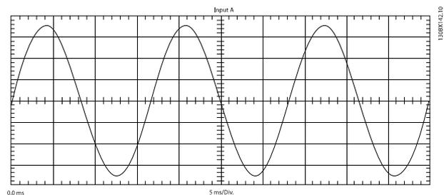
**Illustration 6.15 Normal AC Input Voltage Waveform**
