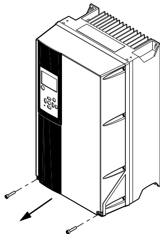
Fig. 23 Access to signal terminals, A4, A5, B1, B2, B3, B4, C1, C2, C3 and C4
