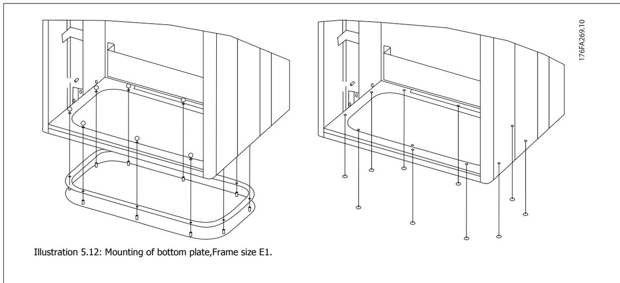
The bottom plate of the E1 frame can be mounted from either in- or outside of the enclosure, allowing flexibility in the installation process, i.e. if mounted from the bottom the glands and cables can be mounted before the frequency converter is placed on the pedestal.
