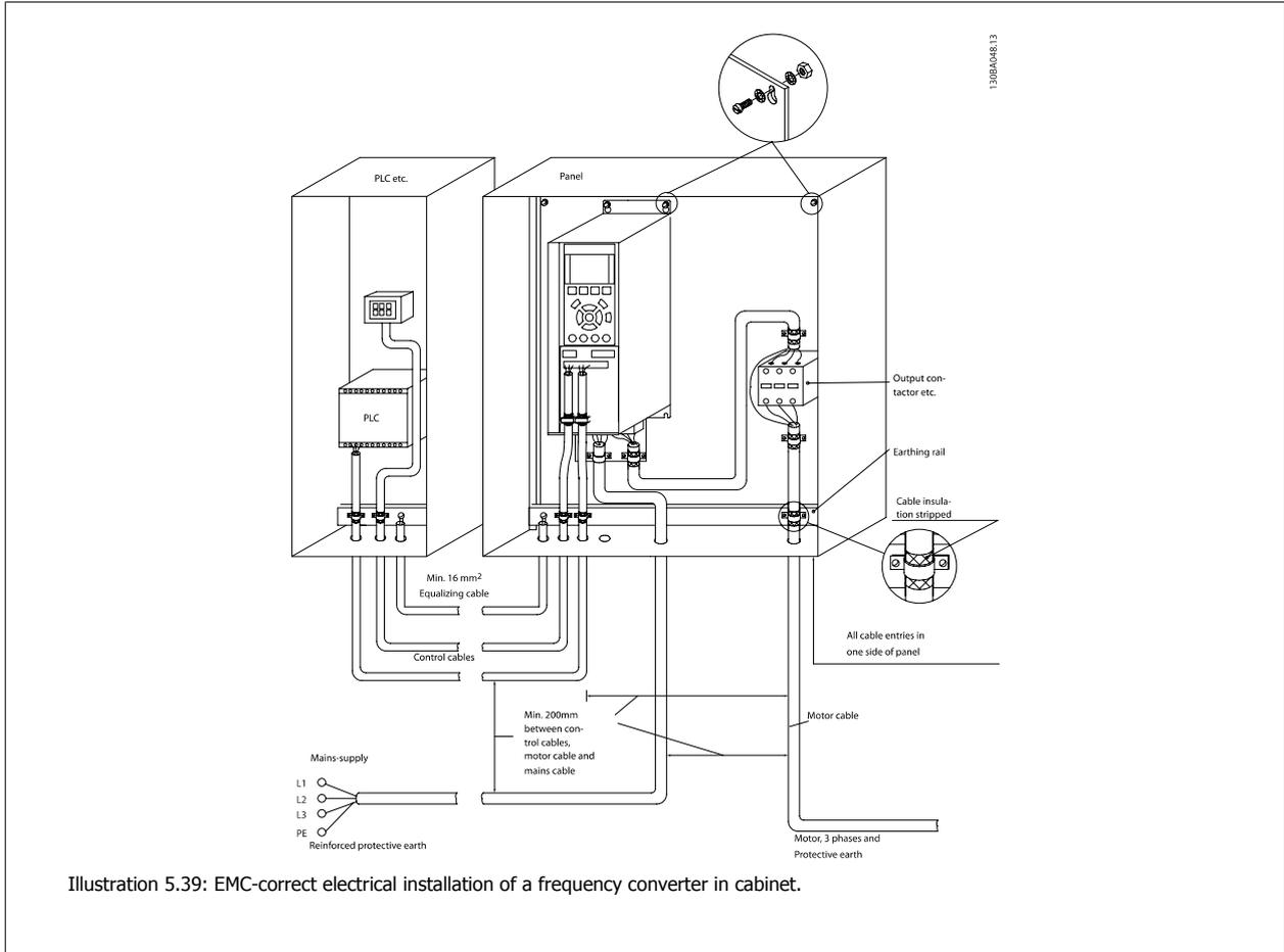
Illustration 5.39: EMC-correct electrical installation of a frequency converter in cabinet.
