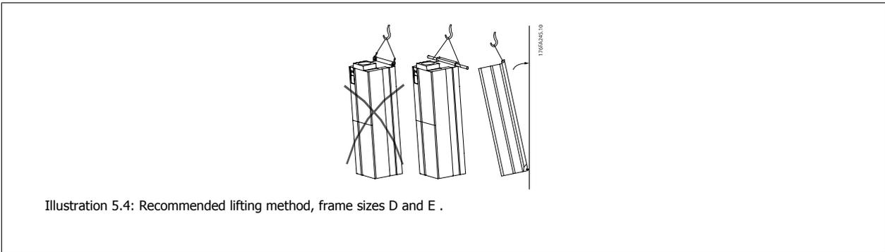
Illustration 5.4: Recommended lifting method, frame sizes D and E .
