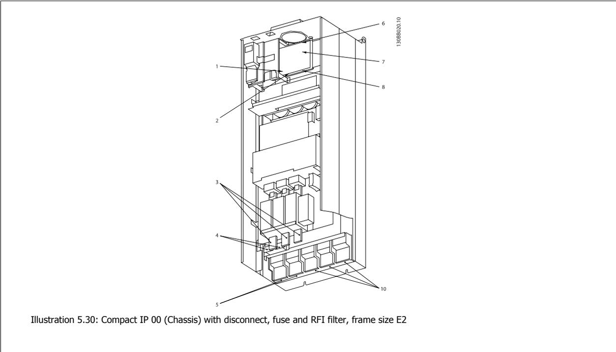
Illustration 5.30: Compact IP 00 (Chassis) with disconnect, fuse and RFI filter, frame size E2
