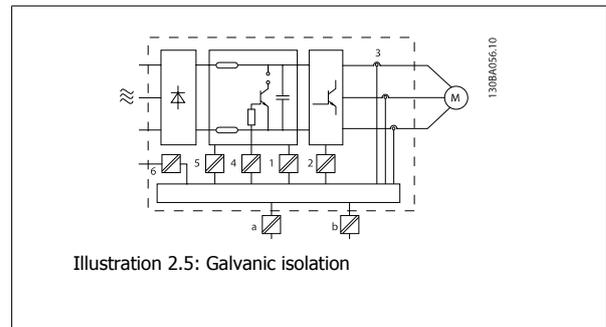
The functional galvanic isolation (a and b on drawing) is for the 24 V back-up option and for the RS 485 standard bus interface.
