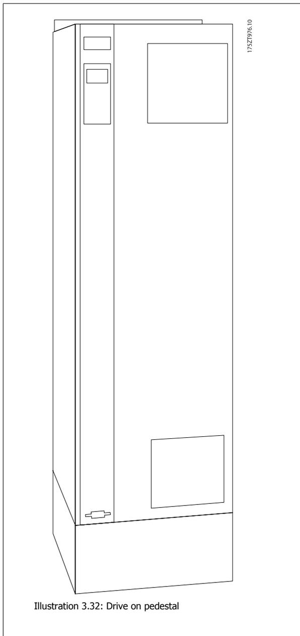
There is one pedestal that fits both frames D1 and D2. Its ordering number is 176F1827. The pedestal is standard for E1 frame.
