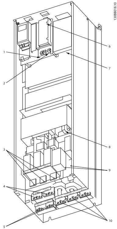
Illustration 5.26: Compact IP 00 (Chassis) with disconnect, fuse and RFI filter, frame size D4
