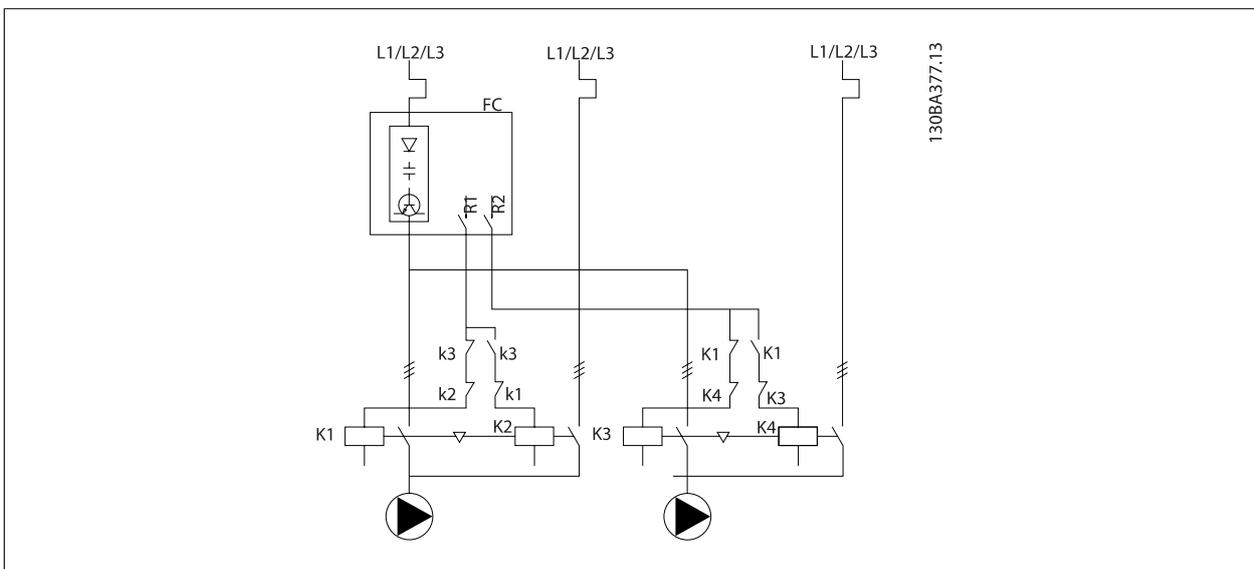
Every pump must be connected to two contactors (K1/K2 and K3/K4) with a mechanical interlock. Thermal relays or other motor protection devices must be applied according to local regulation and/or individual demands.
