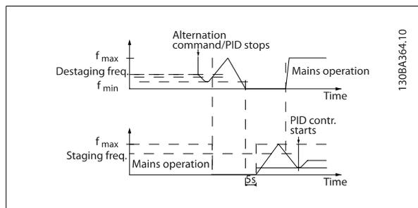
After a time delay, the relay for the fixed speed pump cuts in (staged) and this pump becomes the new lead pump. The new lead pump ramps up to maximum speed and then down to minimum speed. When ramping down and reaching the staging frequency, the old lead pump is now cut in (staged) on the mains as the new fixed speed pump.
