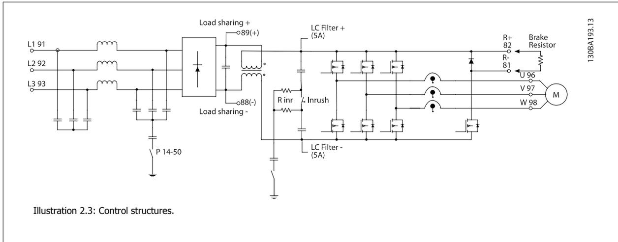
The frequency converter is a high performance unit for demanding applications. It can handle various kinds of motor control principles such as U/f special motor mode and VVC plus and can handle normal squirrel cage asynchronous motors.
