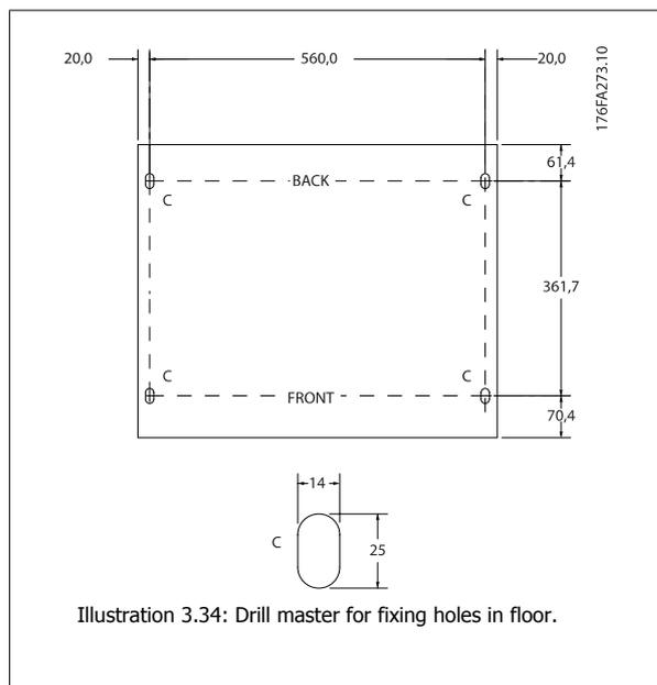
Illustration 3.34: Drill master for fixing holes in floor.
