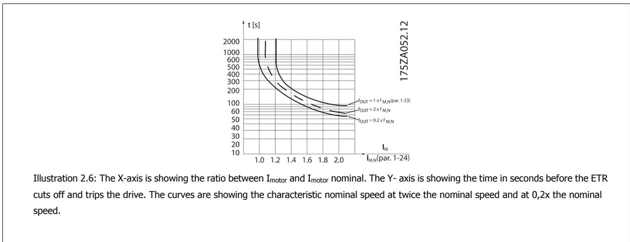
It is clear that at lower speed the ETR cuts of at lower heat due to less cooling of the motor. In that way the motor are protected from being over heated even at low speed. The ETR feature is calculating the motor temperature based on actual current and speed. The calculated temperature is visible as a read out parameter in par. 16-18 *Motor Thermal* in the frequency converter.
