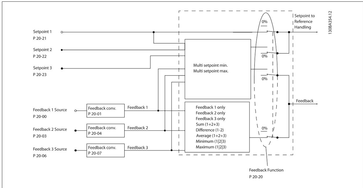
Feedback handling can be configured to work with applications requiring advanced control, such as multiple setpoints and multiple feedbacks. Three types of control are common.
