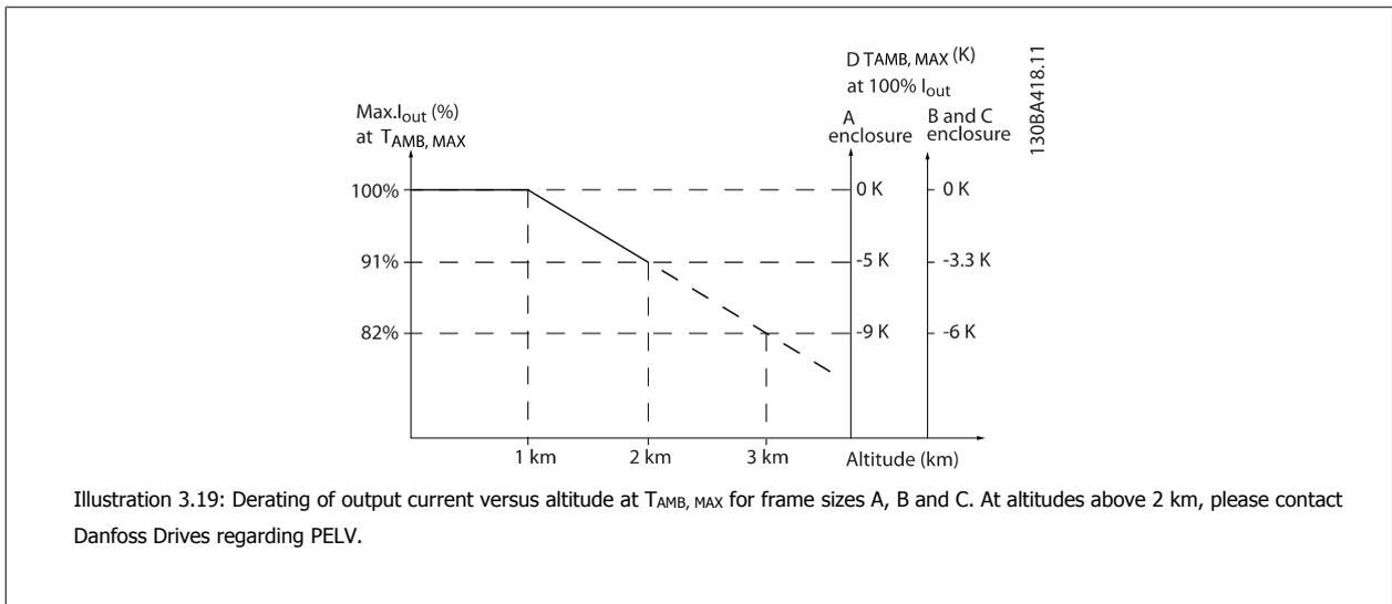
An alternative is to lower the ambient temperature at high altitudes and thereby ensure 100% output current at high altitudes. As an example of how to read the graph, the situation at 2 km is elaborated. At a temperature of 45° C ( $T_{AMB, MAX}$  - 3.3 K), 91% of the rated output current is available. At a temperature of 41.7° C, 100% of the rated output current is available.
