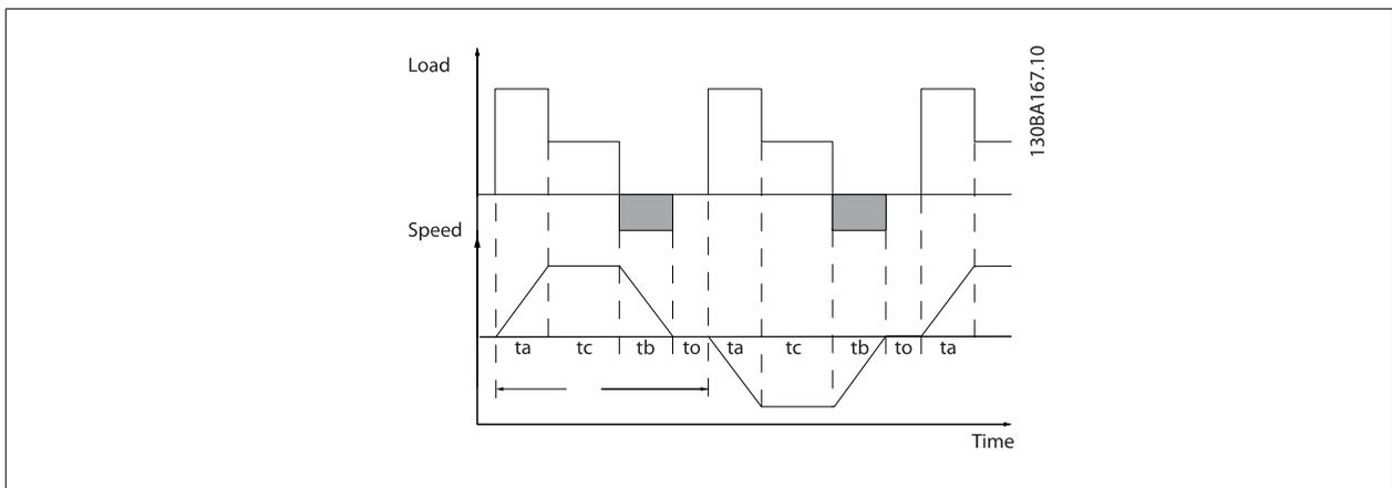
Danfoss offers brake resistors with duty cycle of 5%, 10% and 40% suitable for use with the Automation VT Drive FC322 series. If a 10% duty cycle resistor is applied, this is able of absorbing braking power upto 10% of the cycle time with the remaining 90% being used to dissipate heat from the resistor.
