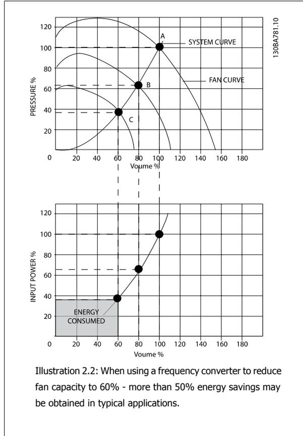
Illustration 2.2: When using a frequency converter to reduce fan capacity to 60% - more than 50% energy savings may be obtained in typical applications.
