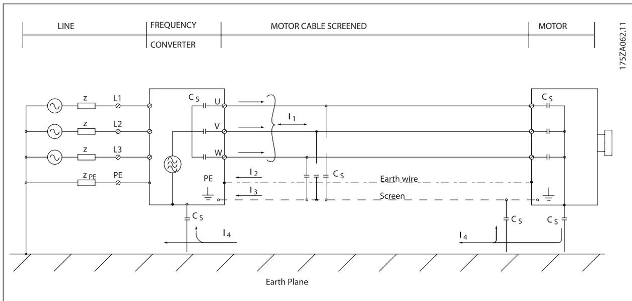
If the screen is to be placed on a mounting plate for the frequency converter, the mounting plate must be made of metal, because the screen currents have to be conveyed back to the unit. Moreover, ensure good electrical contact from the mounting plate through the mounting screws to the frequency converter chassis.
