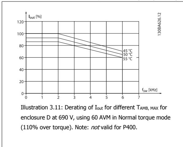
Illustration 3.11: Derating of  $I_{out}$  for different  $T_{AMB, MAX}$  for enclosure D at 690 V, using 60 AVM in Normal torque mode (110% over torque). Note: *not* valid for P400.
