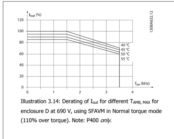
Illustration 3.14: Derating of  $I_{out}$  for different  $T_{AMB, MAX}$  for enclosure D at 690 V, using SFAVM in Normal torque mode (110% over torque). Note: P400 *only*.
