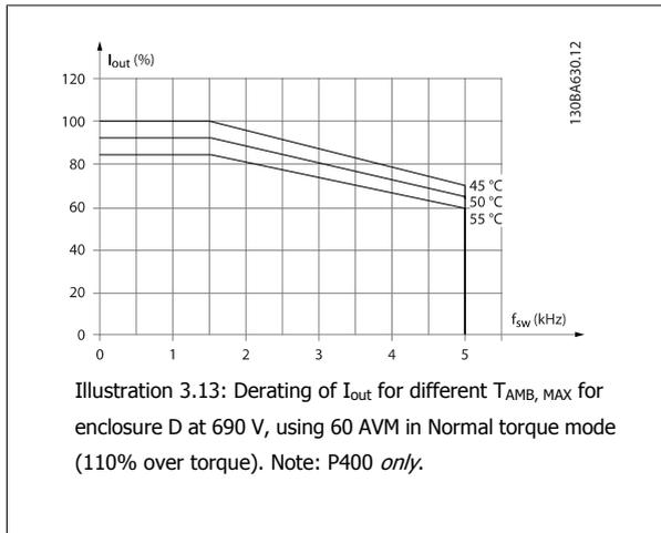
Illustration 3.13: Derating of  $I_{out}$  for different  $T_{AMB, MAX}$  for enclosure D at 690 V, using 60 AVM in Normal torque mode (110% over torque). Note: P400 *only*.
