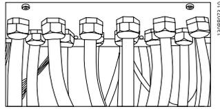
Illustration 5.11: Example of proper installation of the gland plate.
