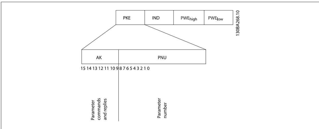
Bits no. 12-15 transfer parameter commands from master to slave and return processed slave responses to the master.
