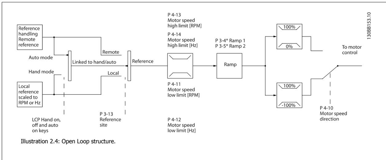
In the configuration shown in the illustration above, *par. 1-00 Configuration Mode* is set to Open loop [0]. The resulting reference from the reference handling system or the local reference is received and fed through the ramp limitation and speed limitation before being sent to the motor control. The output from the motor control is then limited by the maximum frequency limit.
