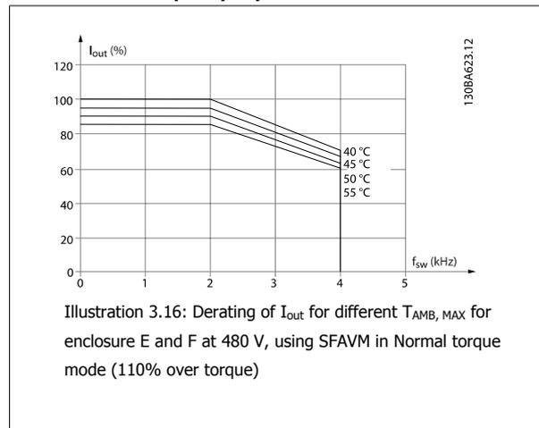
Illustration 3.16: Derating of  $I_{out}$  for different  $T_{AMB, MAX}$  for enclosure E and F at 480 V, using SFAVM in Normal torque mode (110% over torque)
