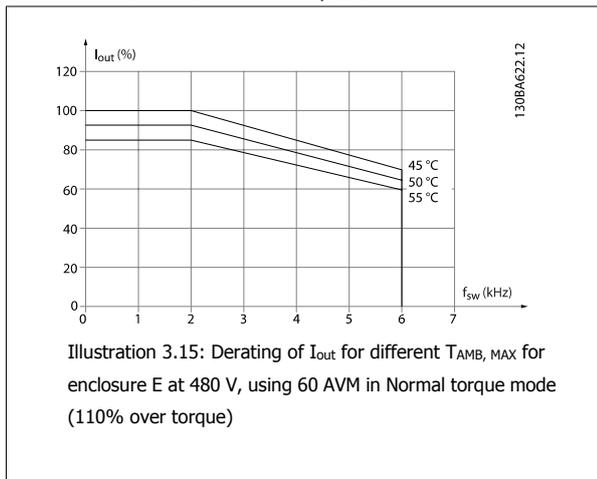
Illustration 3.15: Derating of  $I_{out}$  for different  $T_{AMB, MAX}$  for enclosure E at 480 V, using 60 AVM in Normal torque mode (110% over torque)
