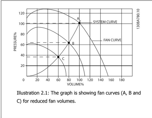
Illustration 2.1: The graph is showing fan curves (A, B and C) for reduced fan volumes.
