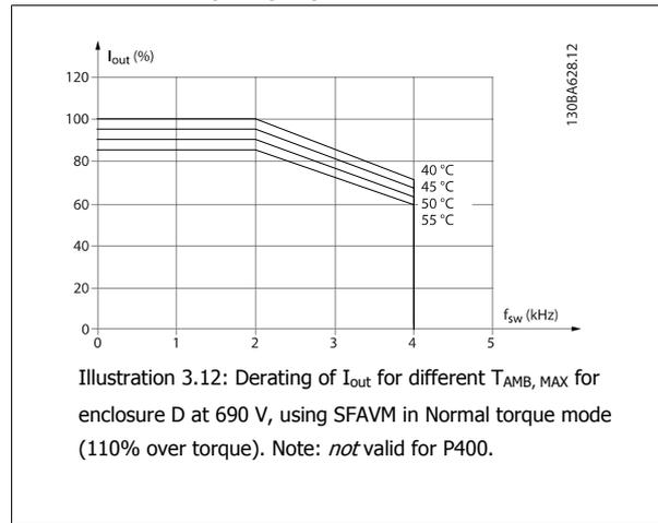
Illustration 3.12: Derating of  $I_{out}$  for different  $T_{AMB, MAX}$  for enclosure D at 690 V, using SFAVM in Normal torque mode (110% over torque). Note: *not* valid for P400.
