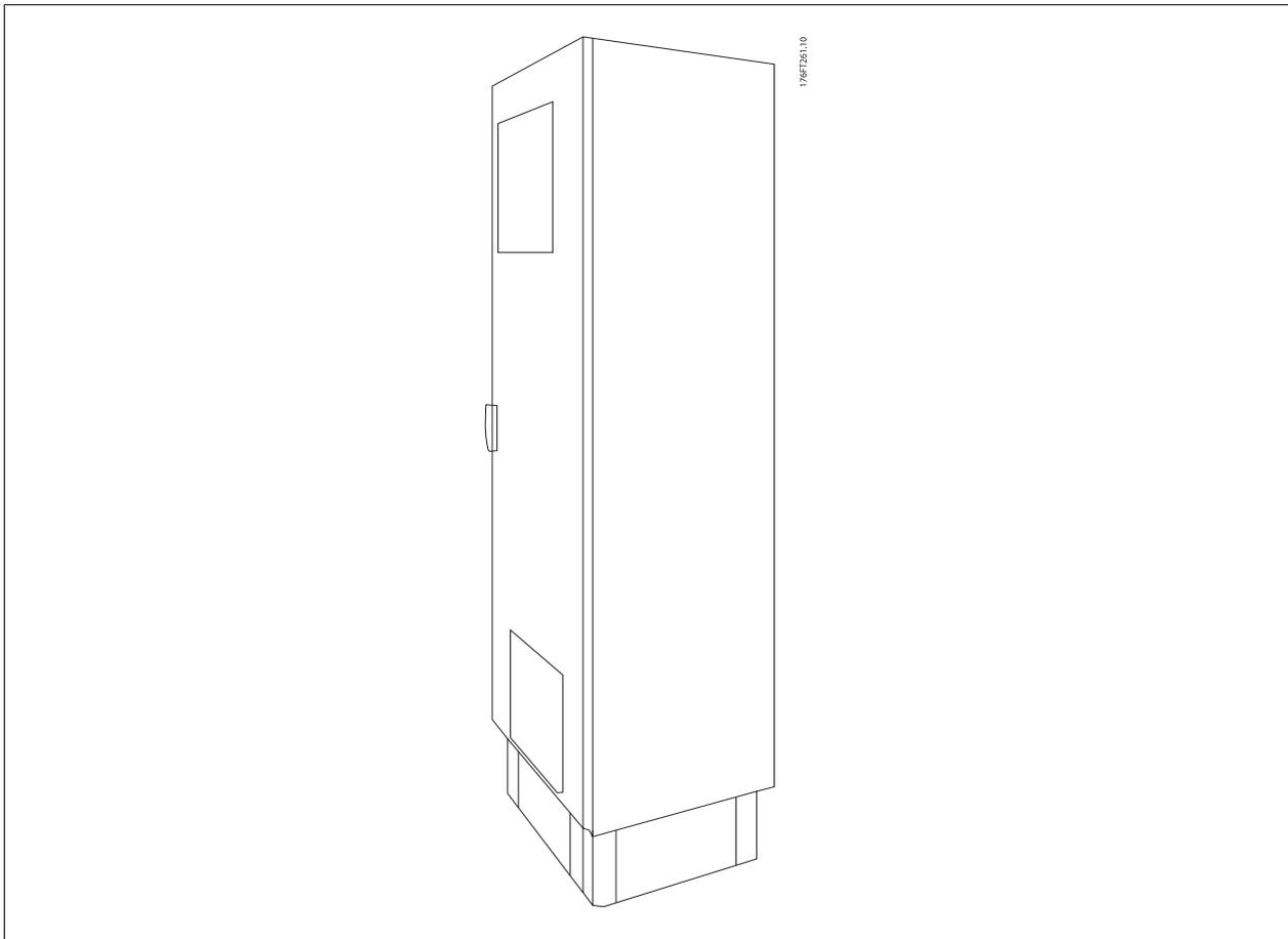
This section is for the installation of NEMA 3R kits available for the frequency converter frames D3, D4 and E2. These kits are designed and tested to be used with IP00/ Chassis versions of these frames in Rittal TS8 NEMA 3R or NEMA 4 enclosures. The NEMA-3R enclosure is an outdoor enclosure that provides a degree of protection against rain and ice. The NEMA-4 enclosure is an outdoor enclosure that provides a greater degree of protection against weather and hosed water.
