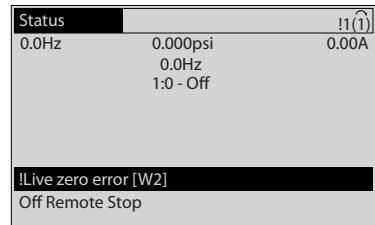
The screenshot shows a digital display interface for a VLT AQUA Drive D. At the top, there's a header with 'Status' and a timestamp '130BP085.11'. Below this is a table with four rows of data: '0.0Hz', '0.000psi', '0.0Hz', and '1:0 - Off'. In the bottom right corner of the display area, there is a black horizontal bar containing the text 'J!Live zero error [W2]' and 'Off Remote Stop'.
