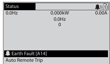
This screenshot shows the same digital display interface as Figure 8.1. It includes the header 'Status' and timestamp '130BP086.11'. The data table shows '0.0Hz', '0.000kW', '0.0Hz', and '0'. In the bottom right corner, there is a black horizontal bar with a bell icon and the text 'Earth Fault [A14]' and 'Auto Remote Trip'.
