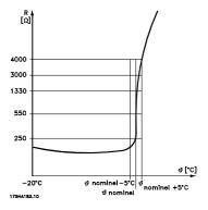
If a motor features a Klixon thermal switch instead, this can also be connected to the input. If motors operate in parallel, the thermistors/thermal switches can be connected in series (total resistance lower than  $3~\mathrm{k}\Omega$ ). Parameter 128 *Motor thermal protection* must be programmed for *Thermistor warning* [1] or *Thermistor trip* [2] and the thermistor is to be connected between a digital input and terminal 50 (+ 10 V supply).
