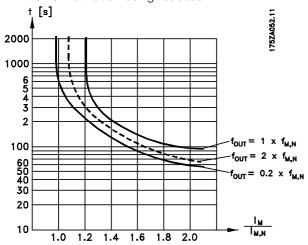
ETR functions 1-4 do not begin to calculate the load until you switch to the Setup in which they have been selected. This means that you can use the ETR function even when changing between two or more motors.
