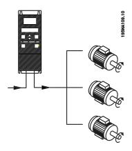
The adjustable frequency drive is able to control several motors connected in parallel. The combined total current consumption of the motors is not to exceed the maximum rated output current (I<sub>INV</sub>) for the adjustable frequency drive. If the motors are to have different rpm values, use motors with different rated rpm values. Motor frequency is changed simultaneously, which means that the ratio between the rated rpm values is maintained.
