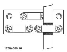
Control wires must be shielded/armored. Connect the shield to the drive chassis with a clamp. Normally, the shield must also be connected to the chassis of the controlling device. (See the instructions for the specific device.) In analog signals or connections using very long wires, 50/60 Hz ground loops may occur because of noise transmitted from the AC line. It may be necessary to break the shield and insert a 100  $\mu\text{F}$ capacitor between the shield and the chassis.
