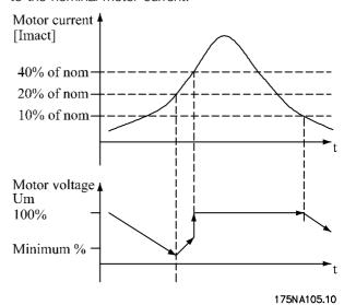
If the active motor current is below 10%, the motor voltage will be decreased by the speed mentioned above until the voltage reaches the setting for Par. 117. If the active motor current comes over 20% the voltage will be increased by the above-mentioned speed. If the active motor current reaches 40% the motor voltage will be increased immediately to normal motor voltage. The reduction in motor voltage depends on the parameter 117 setting.
