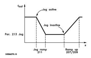
The jog ramp time starts if a jog-signal is given via the LCP control panel, one of the digital inputs or the serial communication port.
