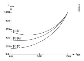
Select Special motor mode [8], if a special U/f setting is needed that is to be adapted to the present motor. The break points are set in parameters 423-428 Voltage/frequency.
