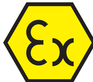
Figure 11.16 ATmosphère EXplosive (ATEX)
