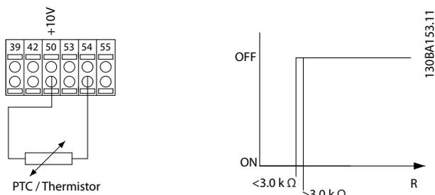
Illustration 3.14 PTC Thermistor Connection - Analog Input
