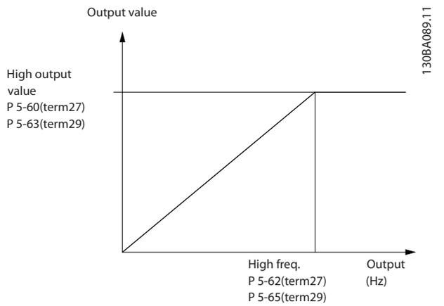
Illustration 3.38 Configuration of Pulse Outputs
