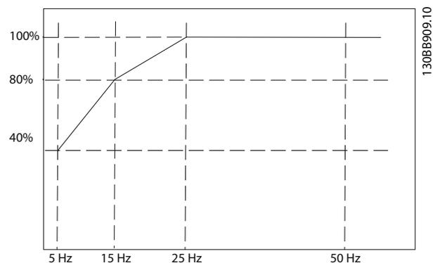
Illustration 3.18 Example of ATEX ETR thermal limitation curve.
