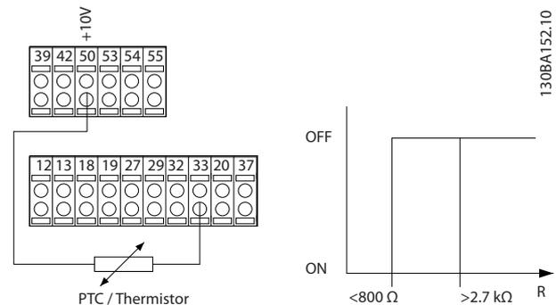
Illustration 3.13 PTC Thermistor Connection - Digital Input
