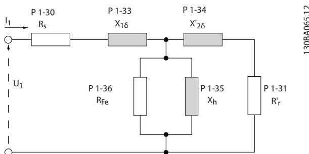
Illustration 3.6 Motor equivalent diagram for an asynchronous motor
