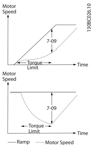
Illustration 3.47 Speed Error between Ramp and Actual Speed
