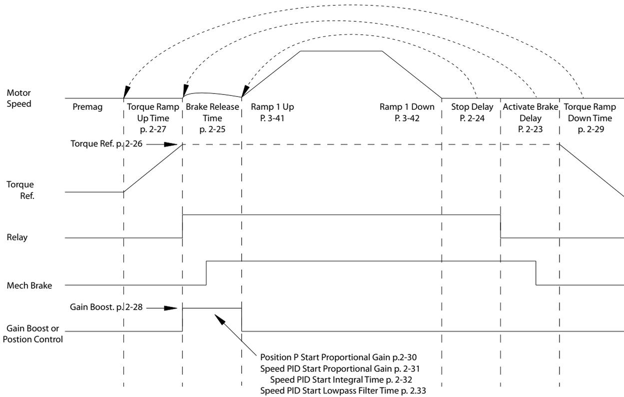
Illustration 3.20 Brake release sequence for hoist mechanical brake control
