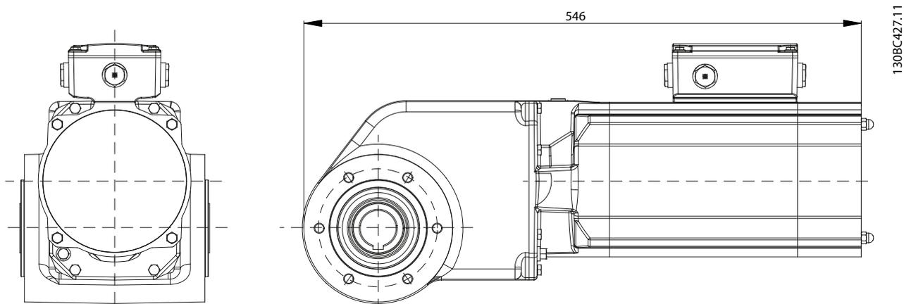
Illustration 8.18 Dimensions: OneGearDrive with Mechanical Brake Option
