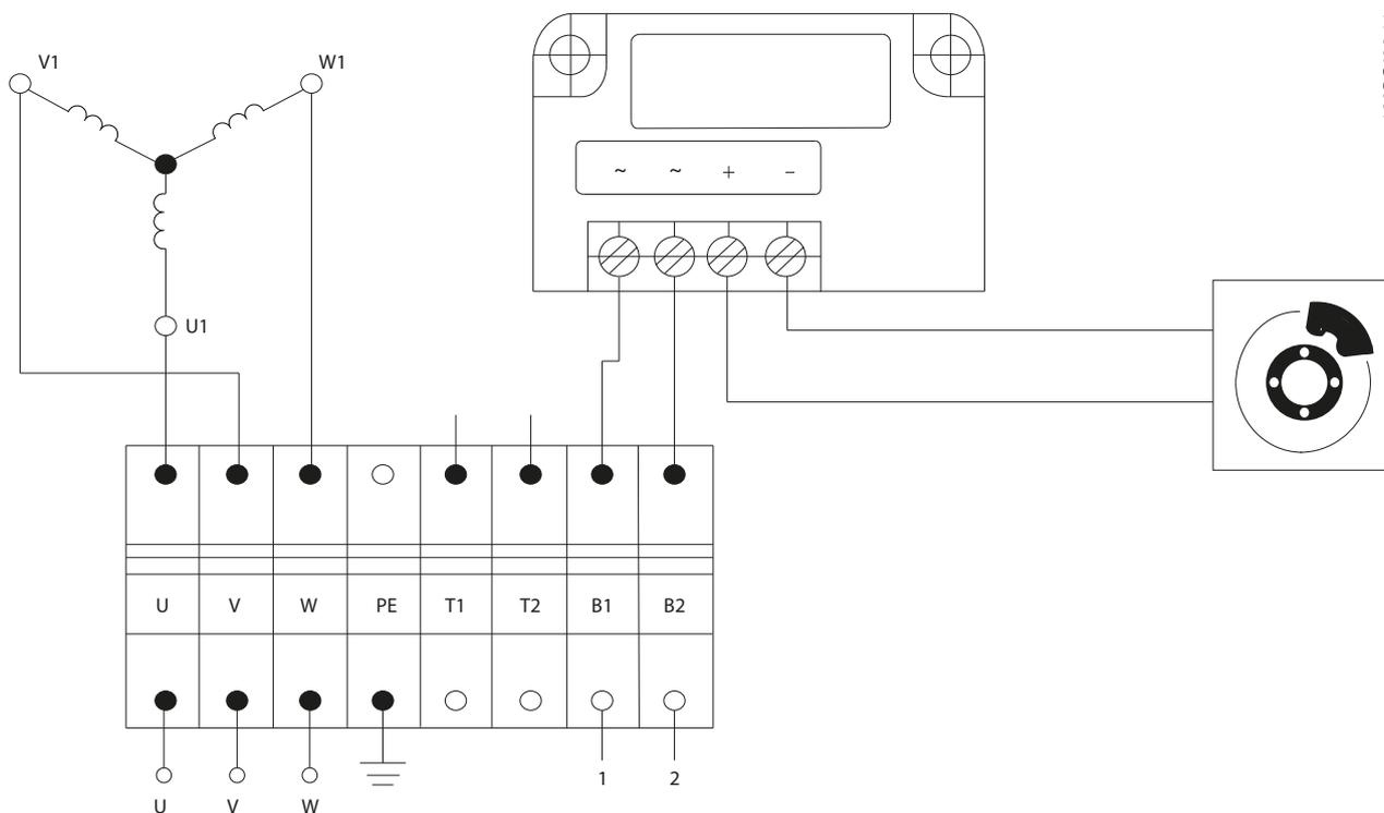
Illustration 8.19 Cage Clamp and Connection to VLT® AutomationDrive FC 302.
