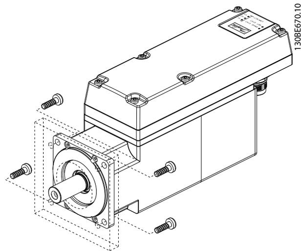
Illustration 4.4 Mounting of Size 1, 1.9 Nm, Size 2, 2.9 Nm, and Size 2, 3.8 Nm Servo Drives
