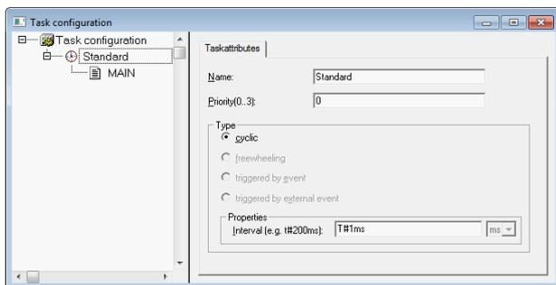
Illustration 6.17 Task Configuration to Parameterize PLC Cycle Time
