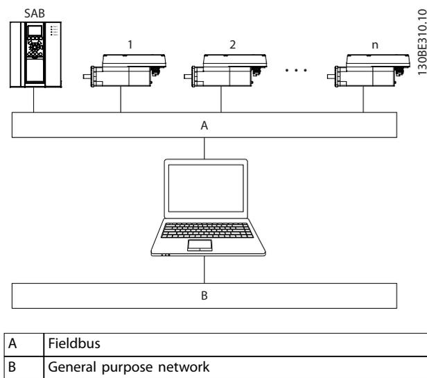
Illustration 6.20 Logical View of Direct Ethernet-based Fieldbus Communication
