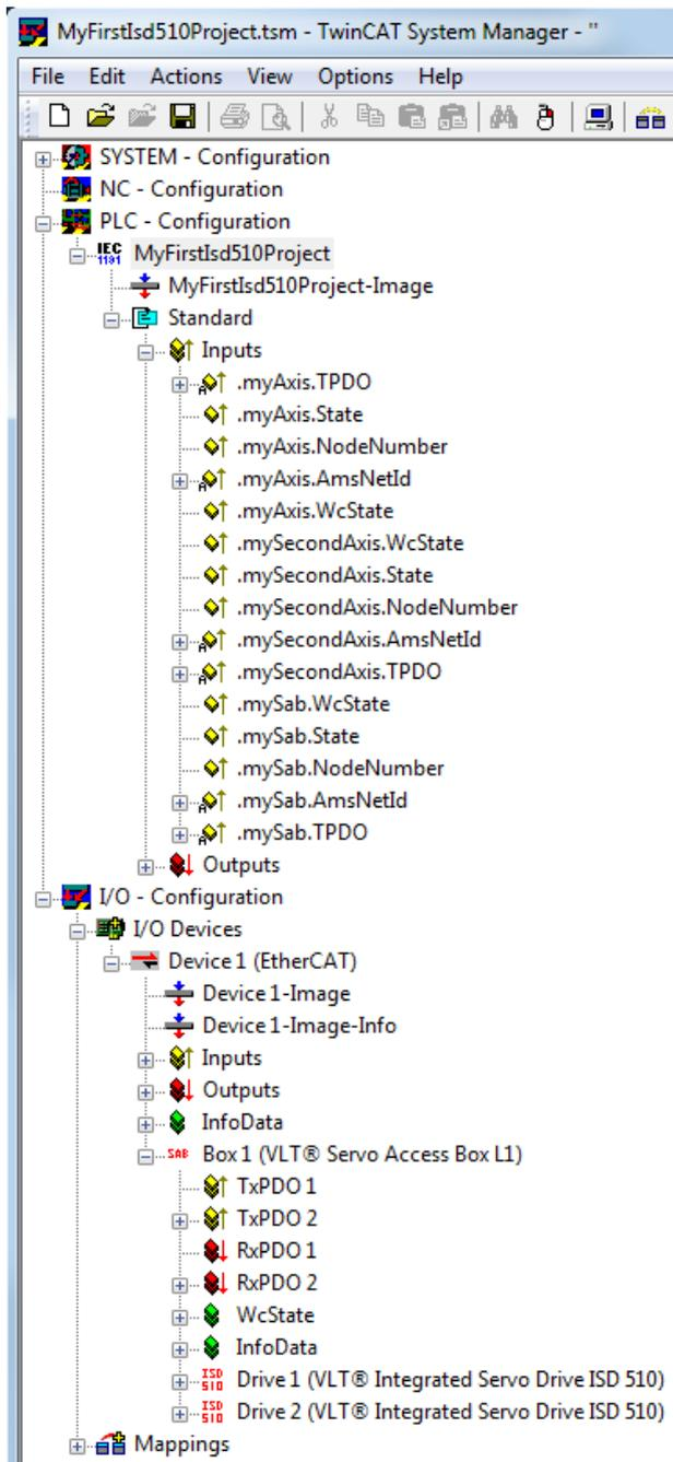
Illustration 6.13 TwinCAT® System Manager after Appending the PLC Project and Adding an SAB and 2 Servo Drives
