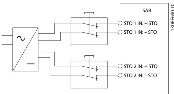
Illustration 8.1 Safety Relay with Plus and Minus Switching Output
