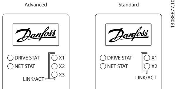
Illustration 7.1 Operating LEDs on the Servo Drive
