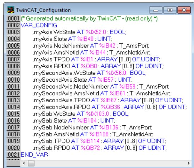
Illustration 6.16 TwinCAT® Configuration: I/O Mapping of 2 Servo Drives and an SAB
