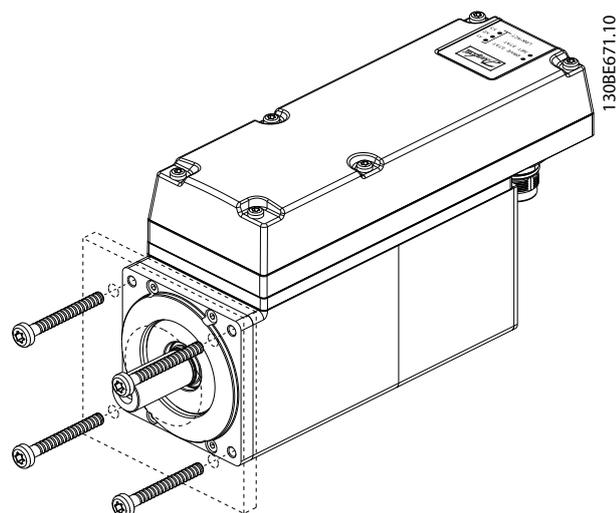
Illustration 4.5 Mounting of Size 2, 2.1 Nm Servo Drive
