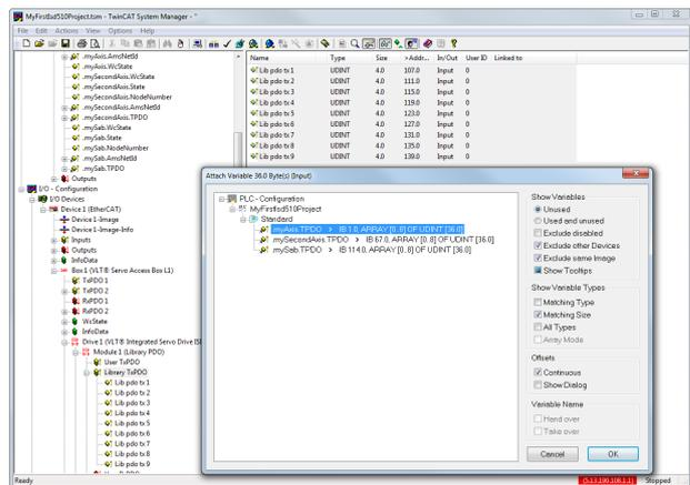
Illustration 6.14 ISD 510 Servo Drive with Correct I/O Configuration
