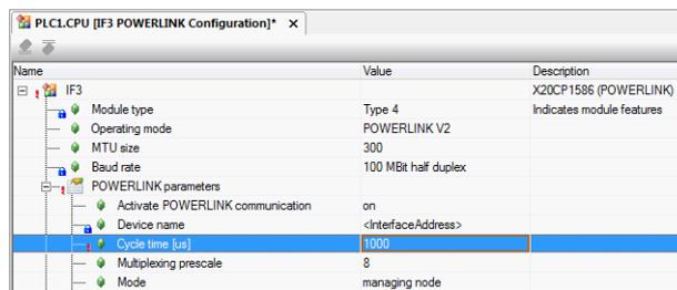
Illustration 6.8 Ethernet POWERLINK® Configuration Window to Parameterize Ethernet POWERLINK® Cycle Time
