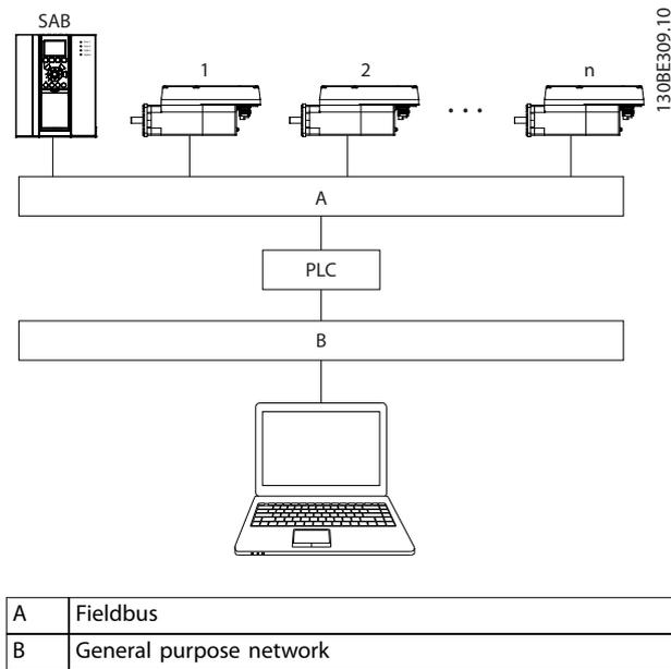
Illustration 6.19 Logical View of Indirect Ethernet-based Fieldbus Communication (Communication via PLC)
