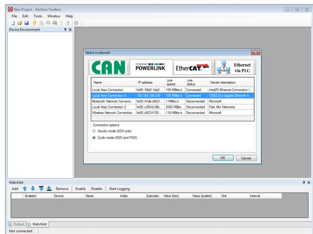
Illustration 6.25 Connect To Network Window (Ethernet POWERLINK®)
