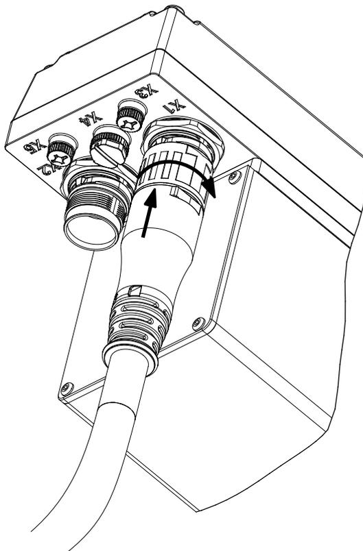
Illustration 5.7 Connecting the M23 Feed-In Cable
