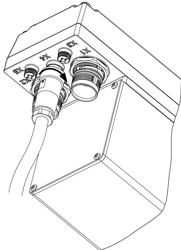
Illustration 5.10 Connecting the I/O and/or Encoder Cable
