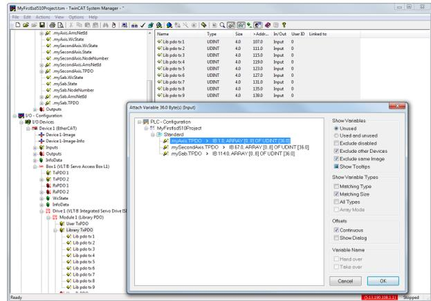
Illustration 6.15 Attaching Inputs and Outputs to the Physical Data Points
