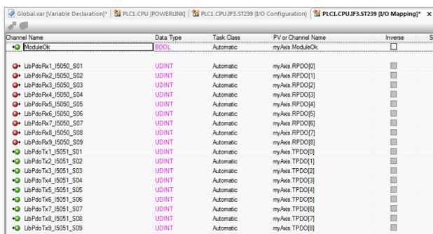
Illustration 6.7 I/O Mapping of an ISD 510 Servo Drive
