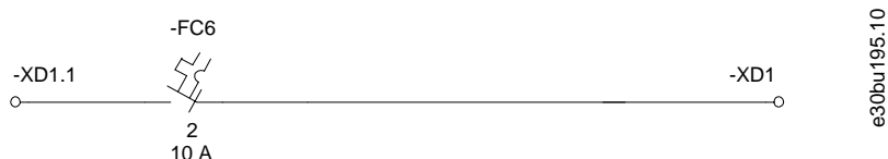
Illustration 42: Auxiliary AC Supply Terminals
