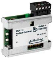
Illustration 3.4 PROFIBUS Converter MCA 114 = 130B1246 (VLT® 5000 = FC 301/302)
