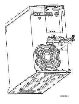
**Step 2**AF-60 LP Micro Drive mounted with de-coupling plate.
