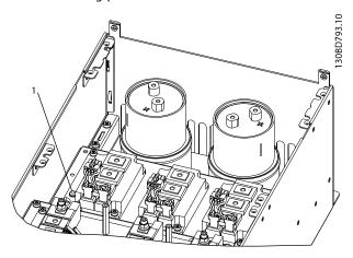
1 Temperature sensor cable connection point
