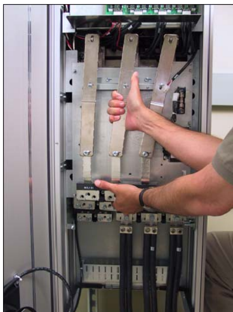
Illustration 2.6 Removing the Existing Input Plate.
