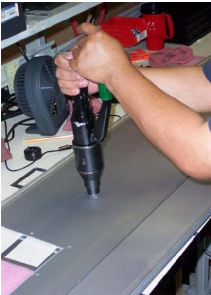
Illustration 4.1 Punching the Disconnect Handle Shaft Hole
