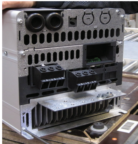
3. Mount the bottom plate again with the four screws and with a torque of 2,5 Nm.
