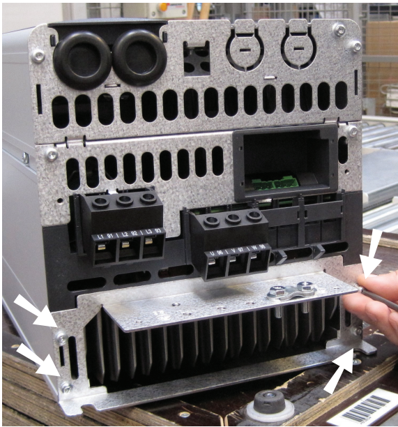
1. Unscrew the four screws indicated with arrows, and remove the plate.
