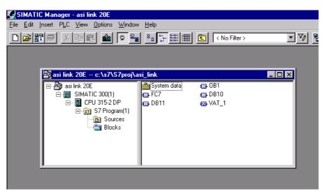
Open Hardware configuration in S7 Manager to configure the system.
