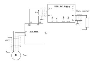
To keep the REEL DC-supply from cutting out for protection when the motor brakes, the resistor Value has to be calculated on the basis of the peak braking power and the intermediate circuit voltage:
