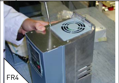
16. Use the attached screws (#5) to fix the IP54 cover on the upper end of the converter.
