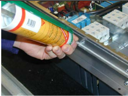
7. Seal the sides of the frequency converter.
