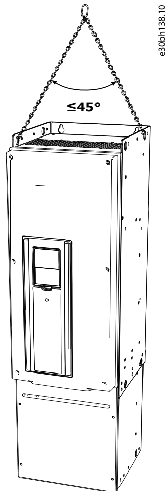
Illustration 2: Maximum Lifting Angle
