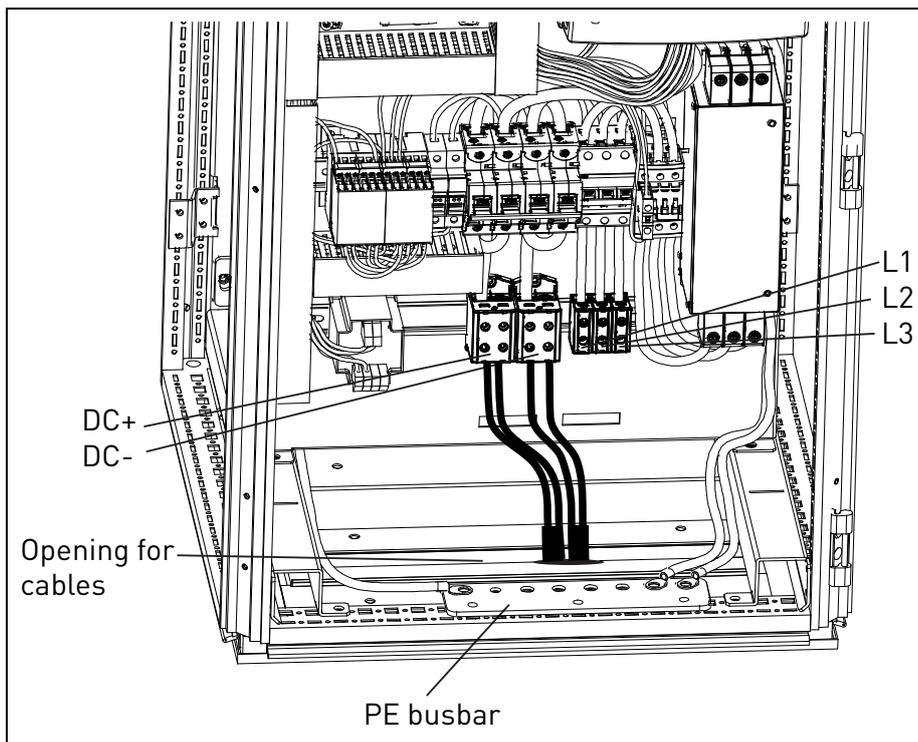
Figure 5-6. Inverter connection to solar panels, NXV0015 to NXV0030
