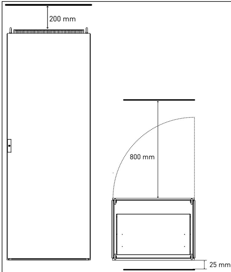
Figure 4-3. Space to be left free above (left) and in front of (right) the cabinet.
