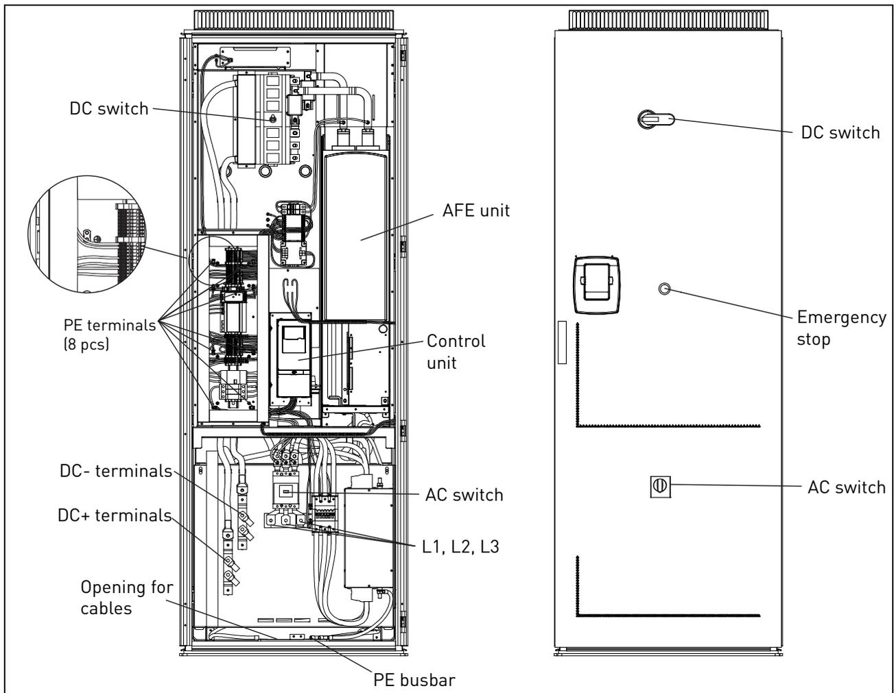
Figure 4-2. Principal drawing of inverter modules NXV0040 and NXV0100 with some essential components
