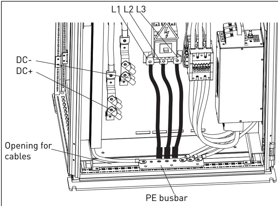
Figure 5-5. Mains cabling NXV0040 and NXV0100 unit (cable clamps not included in delivery)
