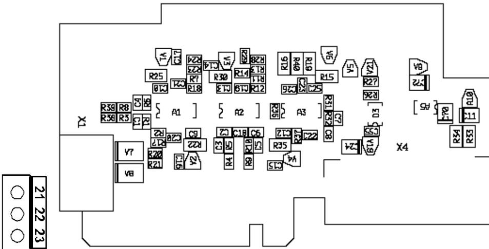
OPTD7 is an AC sinusoidal voltage measurement board. Using this board, the drive measures the line voltage, frequency and voltage angle information. The drive can compare this information with its output voltage angle when running. This feature can be used to develop applications for different purposes using NC61131-3 application programming tool.
