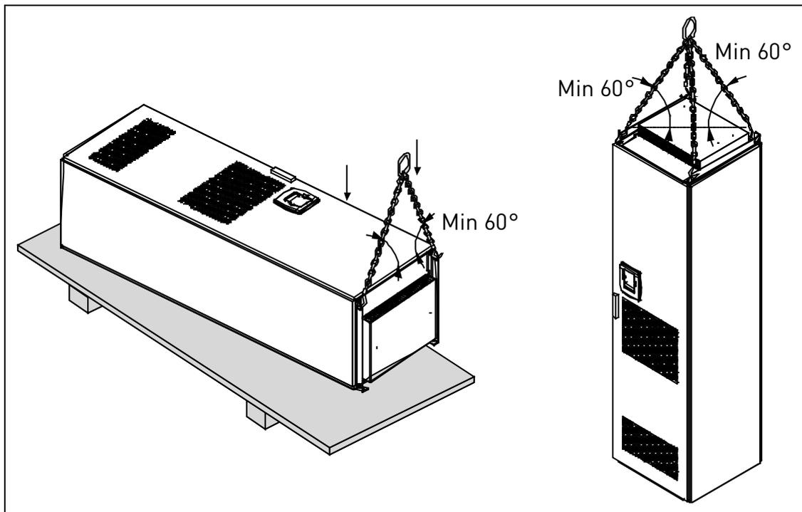
Figure 3-2. Lifting unit cabinet
