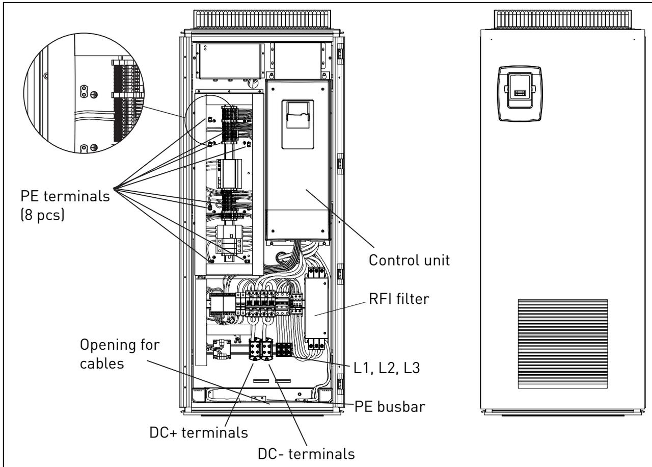
Figure 4-1. Principal drawing of inverter modules NXV0010 to NXV0030 with some essential components
