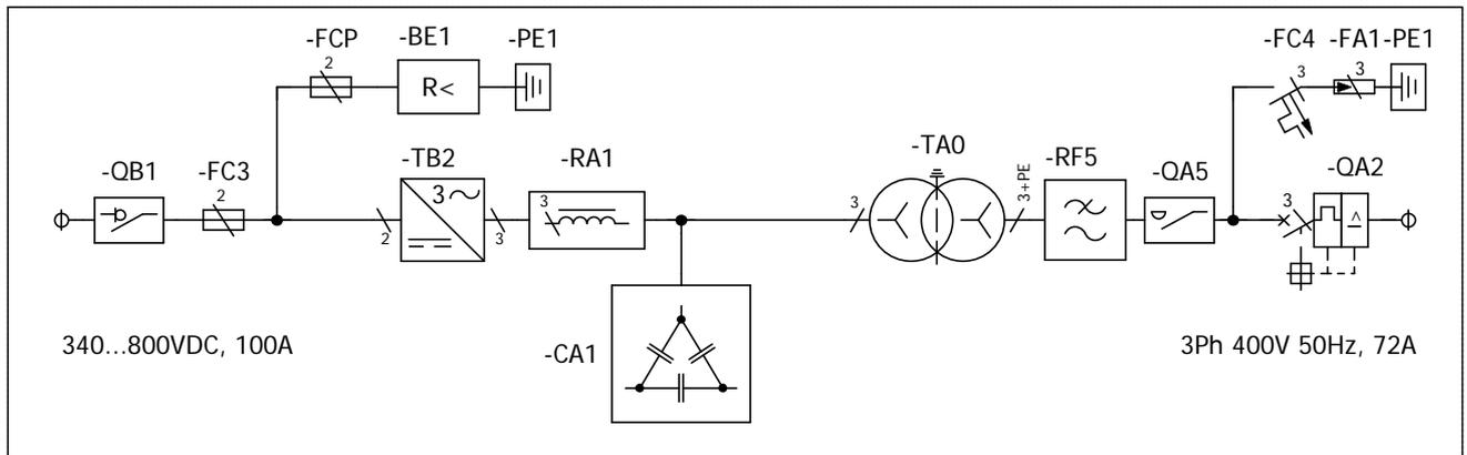
Figure 5-2. Electrical diagram for NXV0040 to NXV0050
