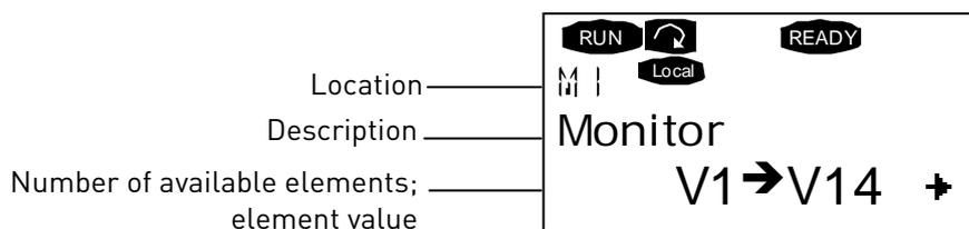
The first menu level has menus from M1 to M7 and it is called *Main menu*. The user can browse the main menu using the Browse push buttons up and down. The chosen submenu can be accessed from the main menu using the Menu push buttons. When there are pages under the menu or page shown, you will see an arrow (➔) in the bottom right corner of the display and you will be able to access the following menu level by pressing the *Push button Menu right*.
