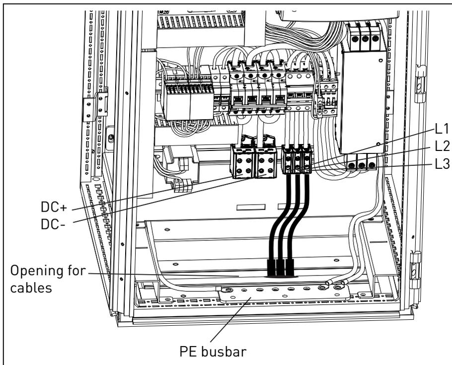
Figure 5-4. Mains cabling NXV0015 to NXV0030 (cable clamps not included in delivery)
