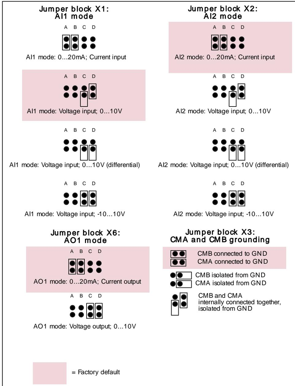
Figure 5-10. Jumper block selection on OPTA1
