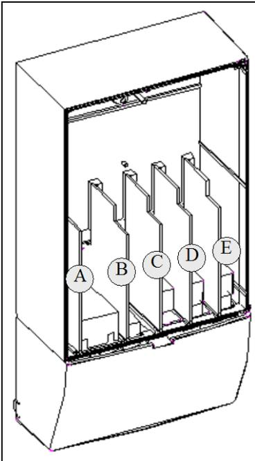
Figure 5-8. Board slots in control unit
