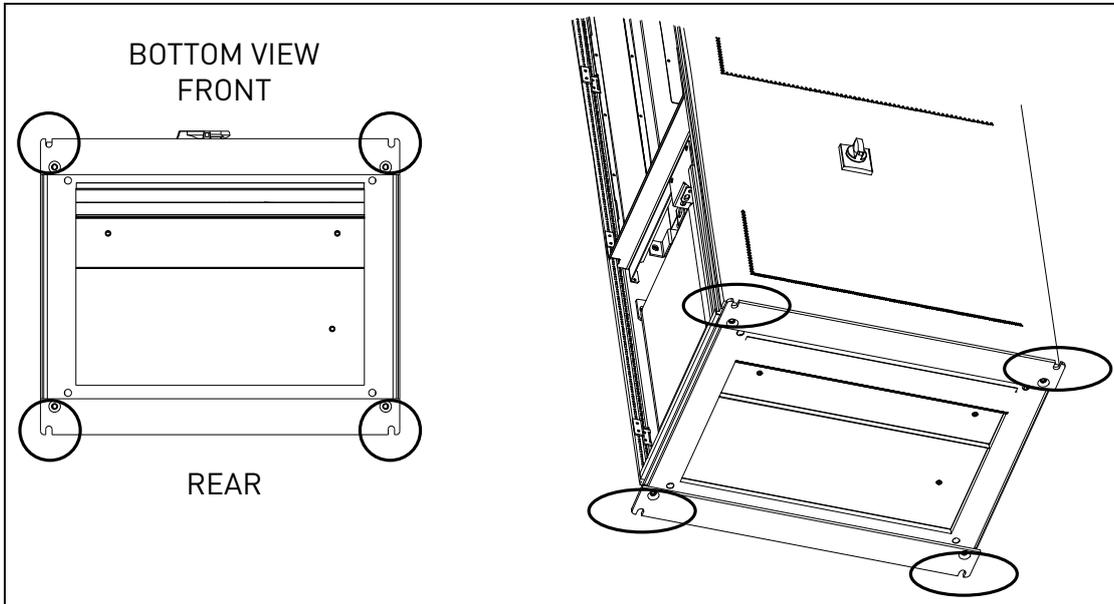
Figure 4-4. Fixing the cabinet to the floor only
