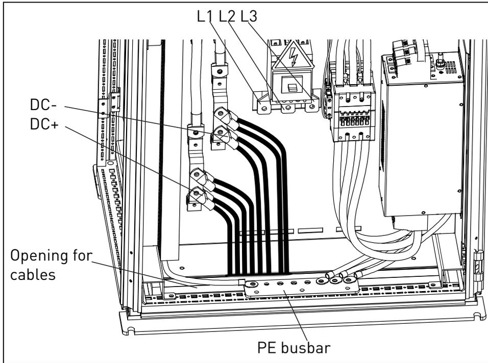
Figure 5-7. Inverter connection to solar panels, NXV0040 to NXV0100
