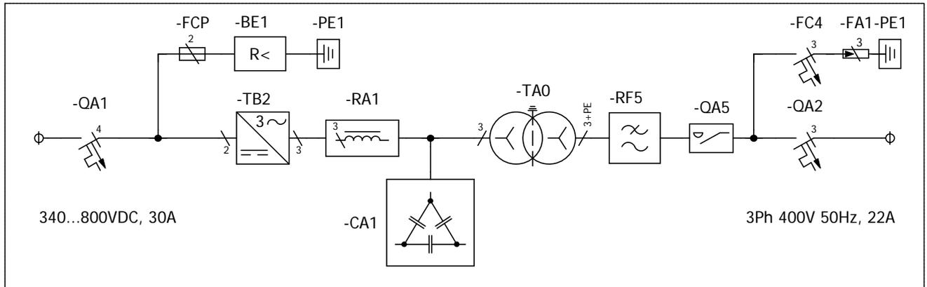
Figure 5-1. Electrical diagram for NXV0010 to NXV0030
