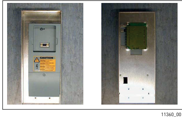
Figure 53. Control unit installed into the mounting box; Left: front; Right: back
