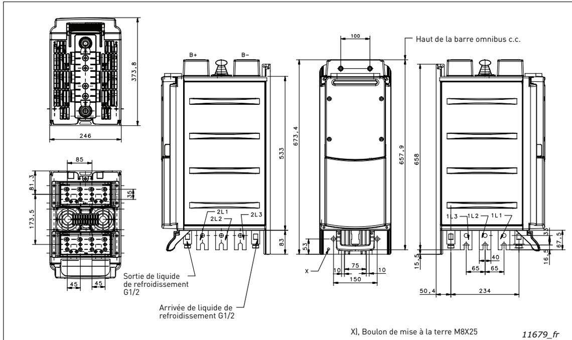
Figure 105. NFE VACON® NXN Liquid-Cooled, CH60
