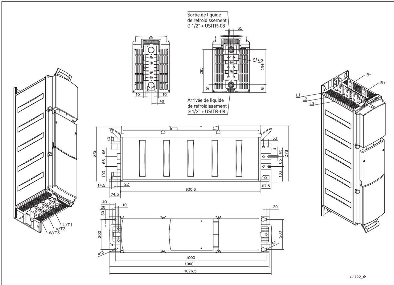
Figure 14. Variateur VACON® Liquid-Cooled (6 impulsions), CH72
