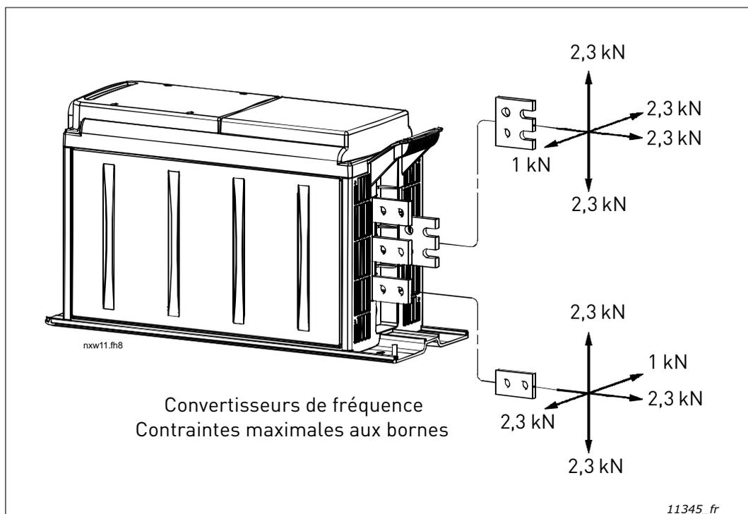
Figure 39. Contraintes maximales aux bornes
