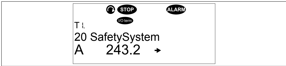
Fig. 73: Fault presentation in the fault lists. The source and fault number are shown as "source.number" (instead of "T1->T16" for other faults).
