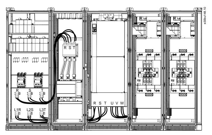
Illustration 40: Connecting Motor and Mains Cables (Example Shows a PHF Cabinet + Input Power Options Cabinet + E6h Drive Cabinet + Sinewave Cabinets)
