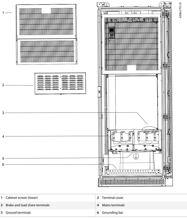
Illustration 49: Connection Points for Mains to Drive Module
