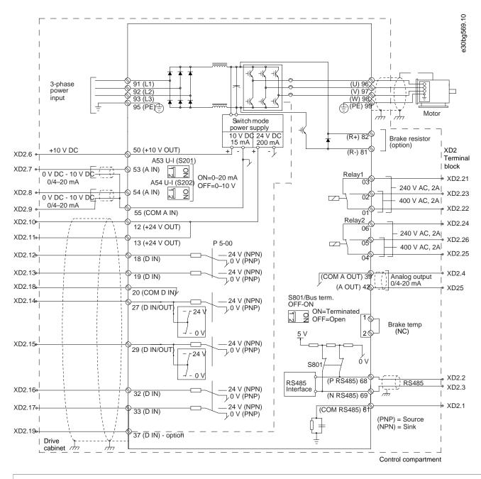
1 Terminal 37 (optional) is used for Safe Torque Off. Refer to the VLT<sup>®</sup> FC Series - Safe Torque Off Operating Guide for installation instructions.
