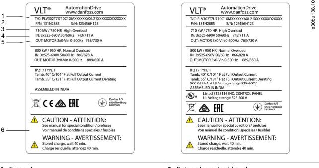
1Type code2Part number and serial number3Power rating4Input voltage, frequency, and current (at low/high voltages)5Output voltage, frequency, and current (at low/high voltages)6
