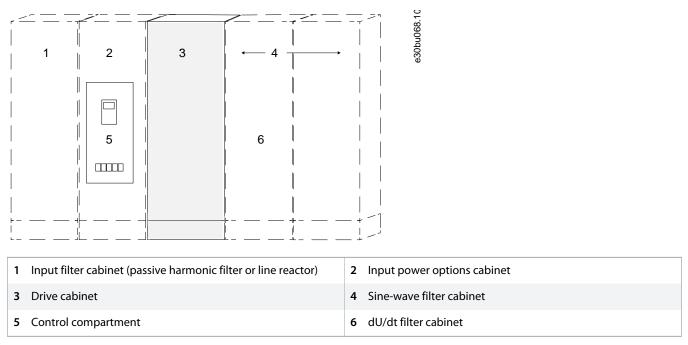
Illustration 3: Possible Configurations for an E5h or E6h Enclosed Drive
