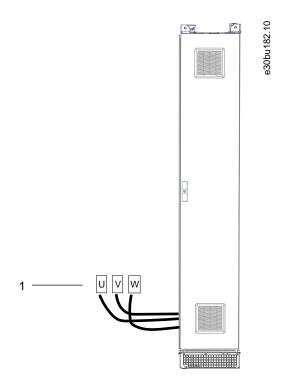
1 Motor cables (U/V/W) to motor terminals (U/V/W) in drive cabinet
