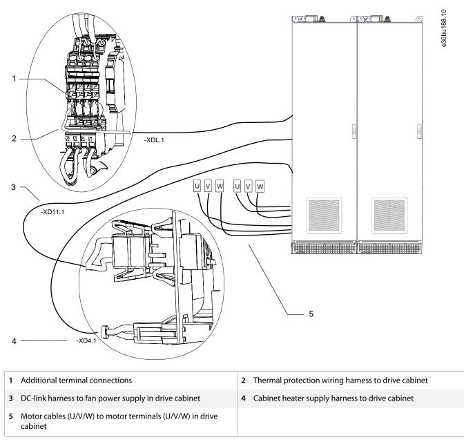
Illustration 37: Split Shipment Electrical Connections (E5h/E6h Sine-wave Cabinets)
