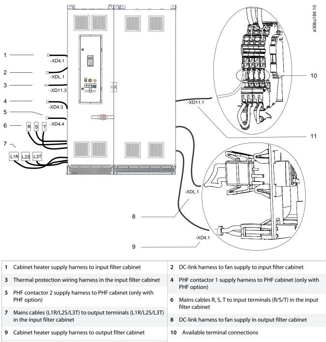
11 Thermal protection wiring harness to output filter cabinet
