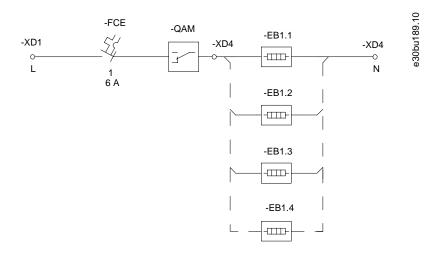
Illustration 47: Motor Heater Control (Heater Element not Included)
