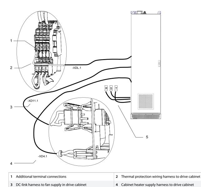
Illustration 27: Split Shipment Electrical Connections (D10h Sine-wave Cabinet)
