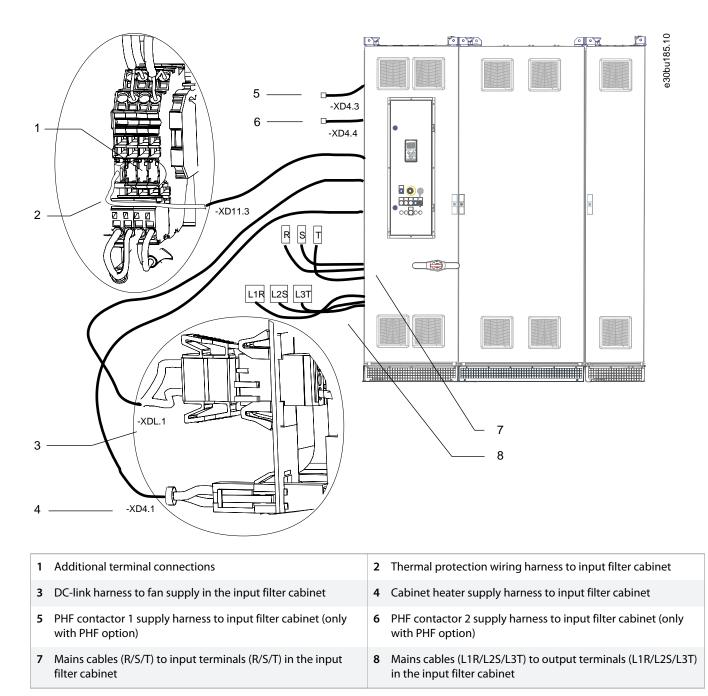
Illustration 38: Split Shipment Electrical Connections (Input Power Options Cabinet + E6h Drive Cabinet + Top Exit Cabinet)
