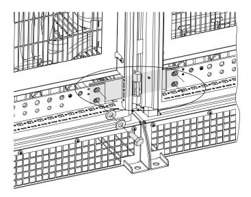
Illustration 16: Connecting the Grounding Bar Between Cabinets
