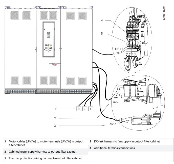
Illustration 32: Split Shipment Electrical Connections (Input Filter Cabinet + Input Power Options Cabinet + E5h Drive Cabinet)
