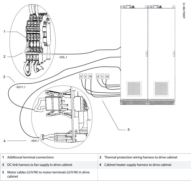
Illustration 31: Split Shipment Electrical Connections (E5h/E6h Sine-wave Cabinets)
