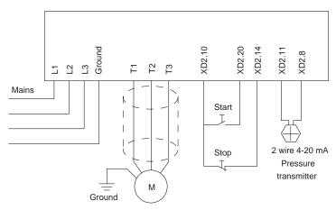
Illustration 63: Wiring for Submersible Pump Application
