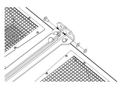
Illustration 15: Connecting the Lifting Eyelet Between Cabinets
