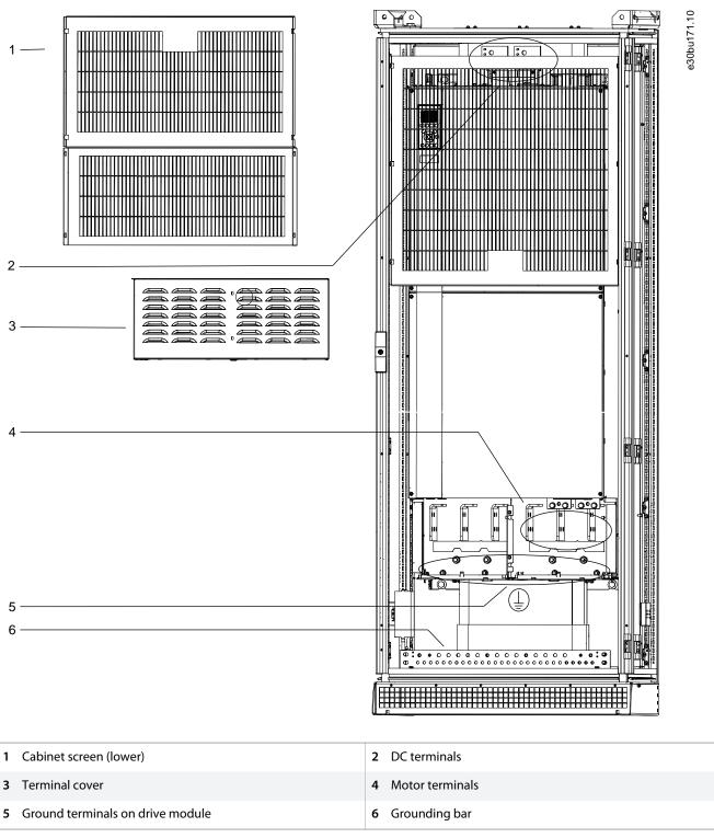
Illustration 52: Connection Points for Drive Module to Motor
