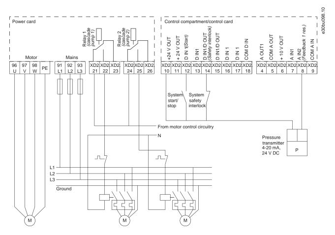
Illustration 65: Cascade Controller Wiring Diagram
