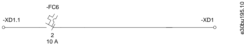
Illustration 41: Auxiliary AC Supply Terminals
