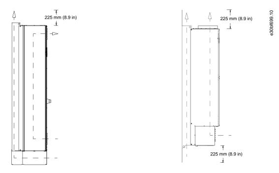
Illustration 68: Airflow for E1h/E2h (Left) and E3h/E4h (Right)
