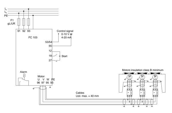
Illustration 43: Speed Control Using Analog Reference (Open Loop) – Single Fan or Pump/Multiple Fans or Pumps in Parallel
