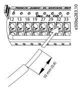
Illustration 35: Connecting a Solid Control Cable to the Terminal Box
