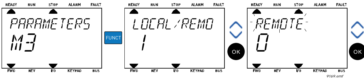
Figure 71. Changing control places.
