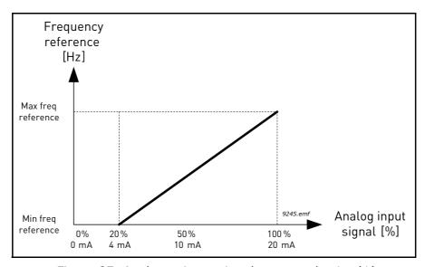
Figure 37. Analogue input signal range, selection '1'
