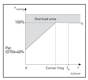
Figure 44. Motor thermal current  $I_T$  curve
