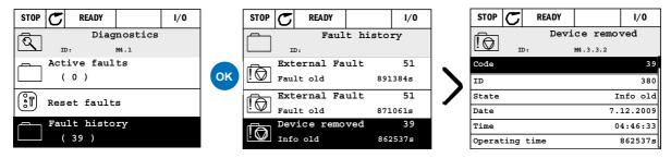
Figure 61. Fault history menu with graphical keypad.
