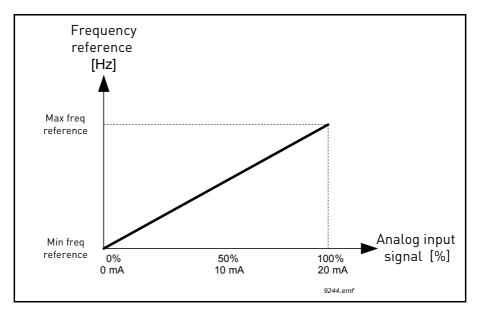
Figure 36. Analogue input signal range, selection '0'
