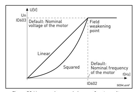
Figure 30.Linear and squared change of motor voltage
