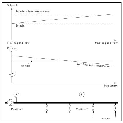
Figure 55. Enable setpoint 1 for pressure loss compensation
