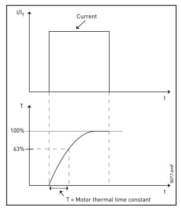
Figure 45. Motor thermal time constant
