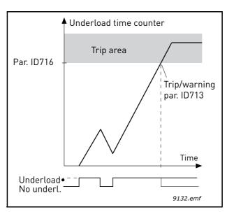
Figure 49. Underload time counter function
