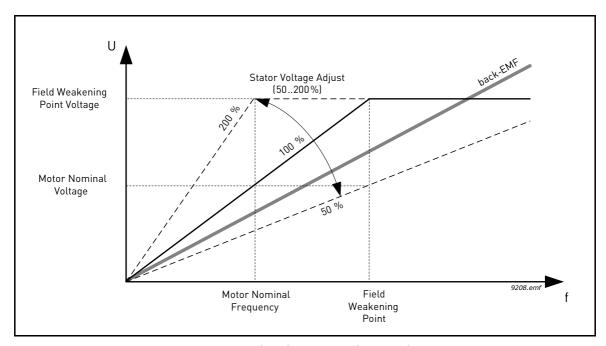
Figure 29. Principle of Stator voltage adjustment
