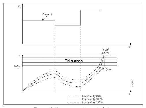
Figure 46. Motor temperature calculation
