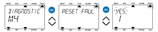
Figure 60. Diagnostic menu with text keypad.
