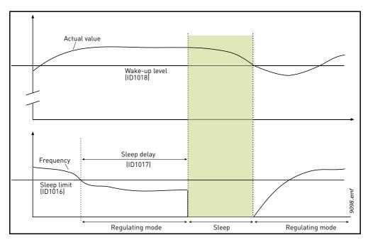
Figure 52. Sleep limit, Sleep delay, Wake-up level
