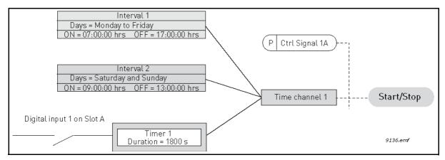
Figure 24. Final configuration where Time channel 1 is used as control signal for start command instead of a digital input.
