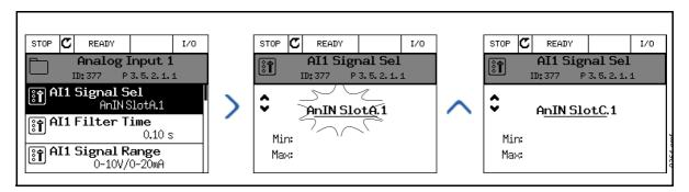
Figure 19. Programming analogue inputs with graphical keypad
