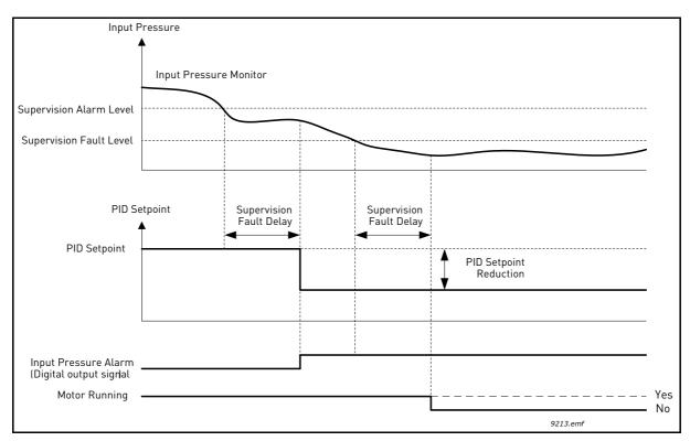
Figure 26. Input pressure supervision.
