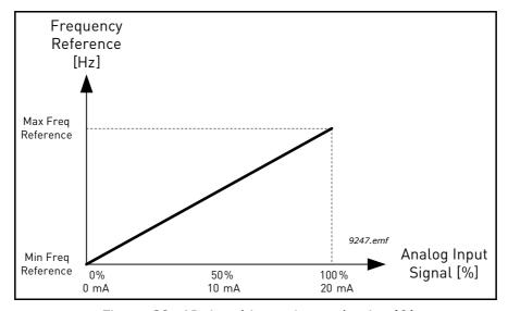
Figure 39. AI signal inversion, selection '0'
