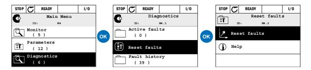
Figure 59. Diagnostic menu with graphical keypad.
