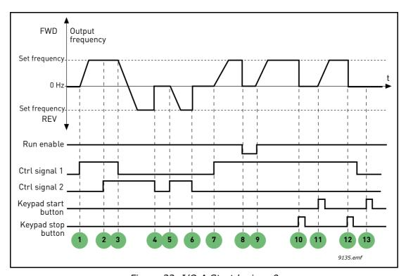
Figure 32. I/O A Start logic = 0
