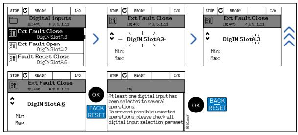
Figure 16. Programming digital inputs with graphical keypad
