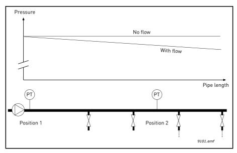
Figure 54. Position of pressure sensor
