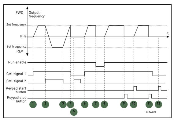
Figure 33. I/O A Start logic = 1
