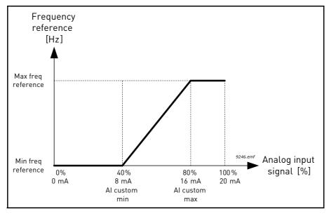
Figure 38. AI signal custom min/max
