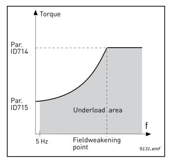
Figure 48. Setting of minimum load
