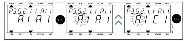
Figure 20. Programming analogue inputs with text keypad
