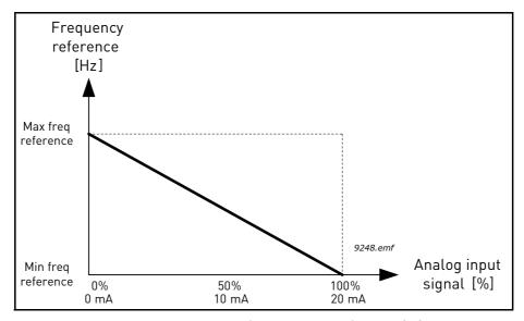
Figure 40. AI signal inversion, selection '1'
