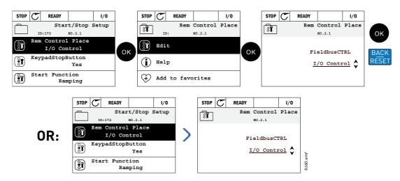
Figure 3. Typical editing of values on graphical keypad (text value)
