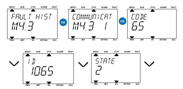
Figure 62. Fault history menu with text keypad.
