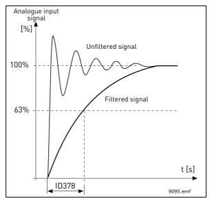
Figure 35. AI1 signal filtering
