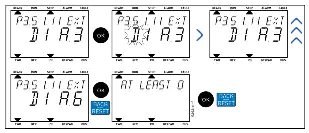
Figure 17. Programming digital inputs with text keypad
