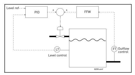
Figure 51. Feedforward control
