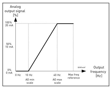
Figure 41. AO1 signal scaling
