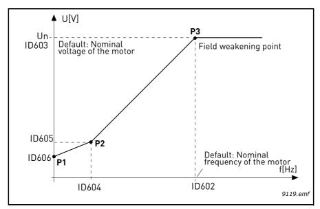
Figure 31.Programmable U/f curve
