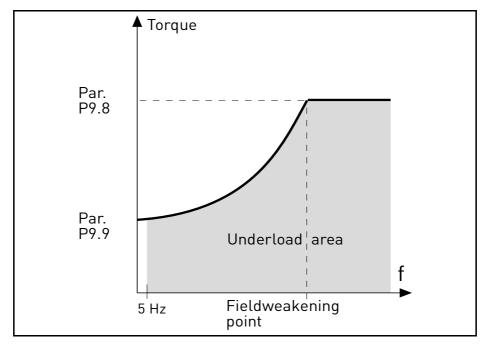
Figure 15. Underload (Dry run) characteristic settings.
