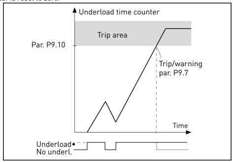
Figure 16. Underload time counter.
