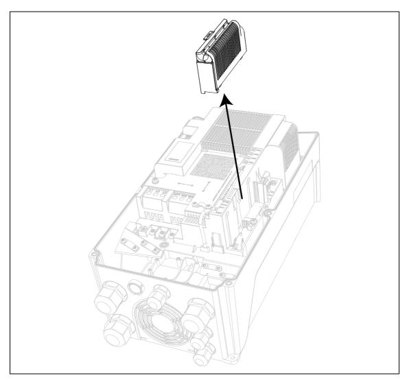
Figure 2. Removing the option slot cover.
