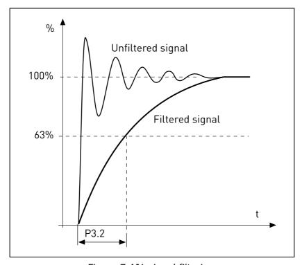
Figure 7.AI1 signal filtering.
