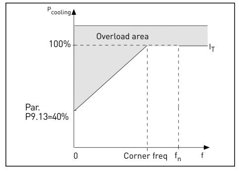
Figure 17. Motor thermal current  $I_T$  curve.
