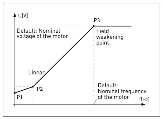
Figure 12. Programmable curve.
