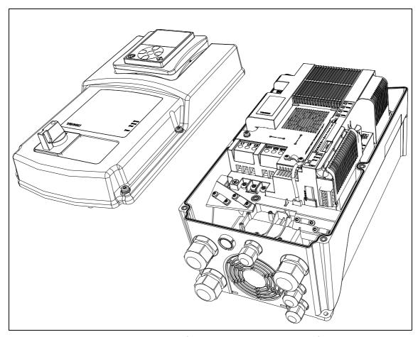
Figure 1. Opening the main cover, MU3 example.
