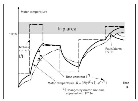
Figure 18. Motor temperature calculation.
