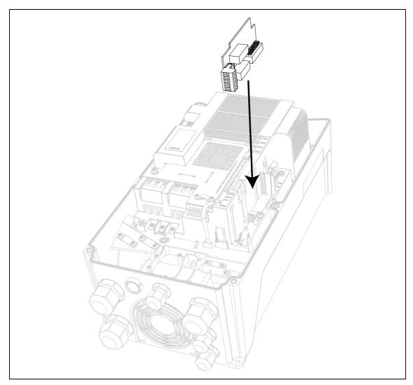
Figure 3. Option board installation.
